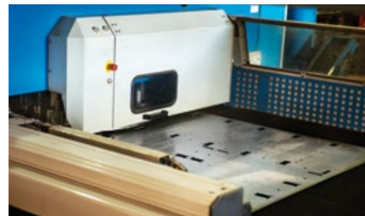
en Sheet punching and bending. The entire process is robotised.
