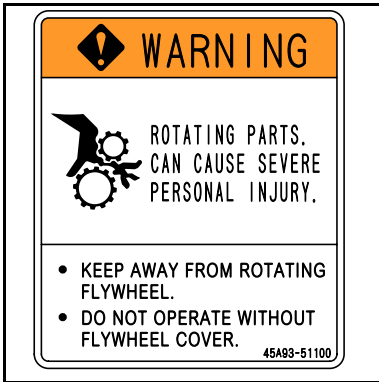
fig.1-1 Warning for flywheel entanglement
