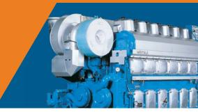
The Wärtsilä 20DF is a four-stroke dual-fuel engine that can be run on natural gas, marine diesel oil (MDO) or heavy fuel oil (HFO). The engine can switch over from gas to MDO/HFO and vice versa smoothly during engine operation without power interruption. The Wärtsilä 20DF design is based on the well proven and reliable Wärtsilä 20 diesel engine which was introduced on the market in the early 1990s. Wärtsilä 20DF completes the lower power range in the dual-fuel Wärtsilä engine family.
