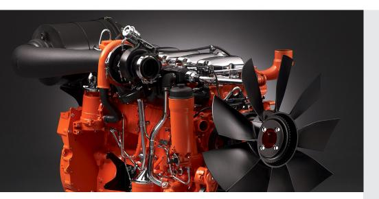
The engines for power generation from Scania are based on a robust design with a strength optimised cylinder block containing wet cylinder liners that can easily be exchanged. Individual cylinder heads with 4 valves per cylinder promotes repairability and fuel economy.
