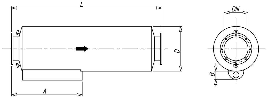
Fig 10-7 Exhaust gas silencer (4V49E0137b)
