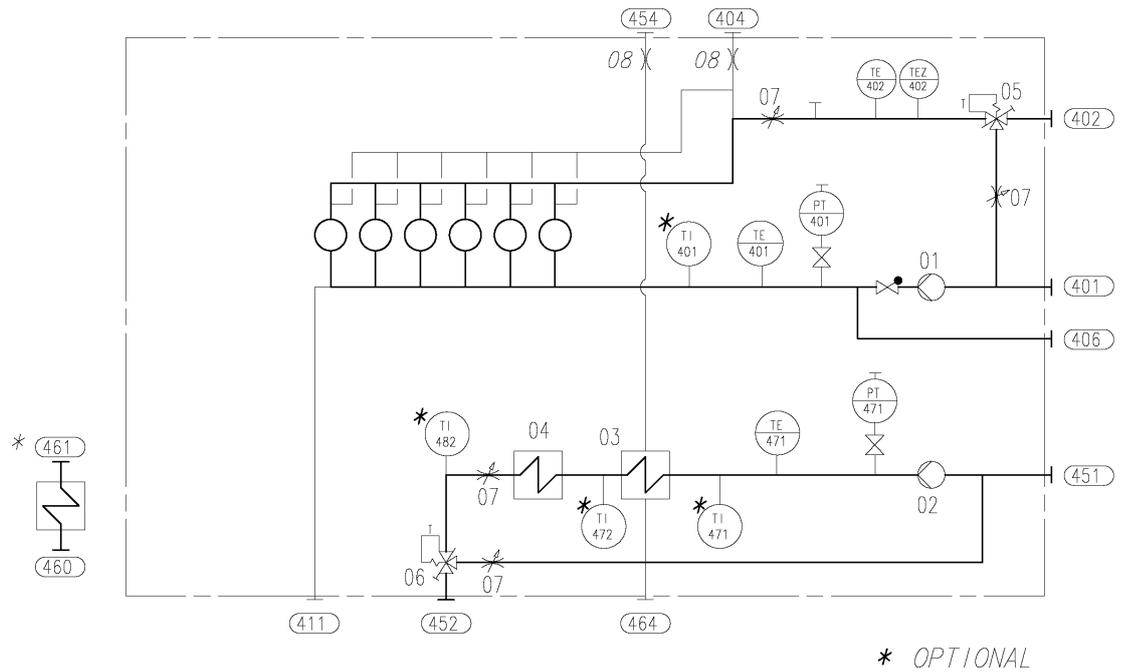
**Fig 8-2 Internal cooling water system, WA20, separate HT and LT (DAAE010162G)**
