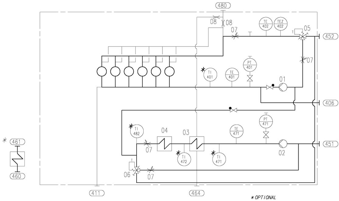
**Fig 8-3 Internal cooling water system, WA20, combined HT and LT (DAAE010159G)**
