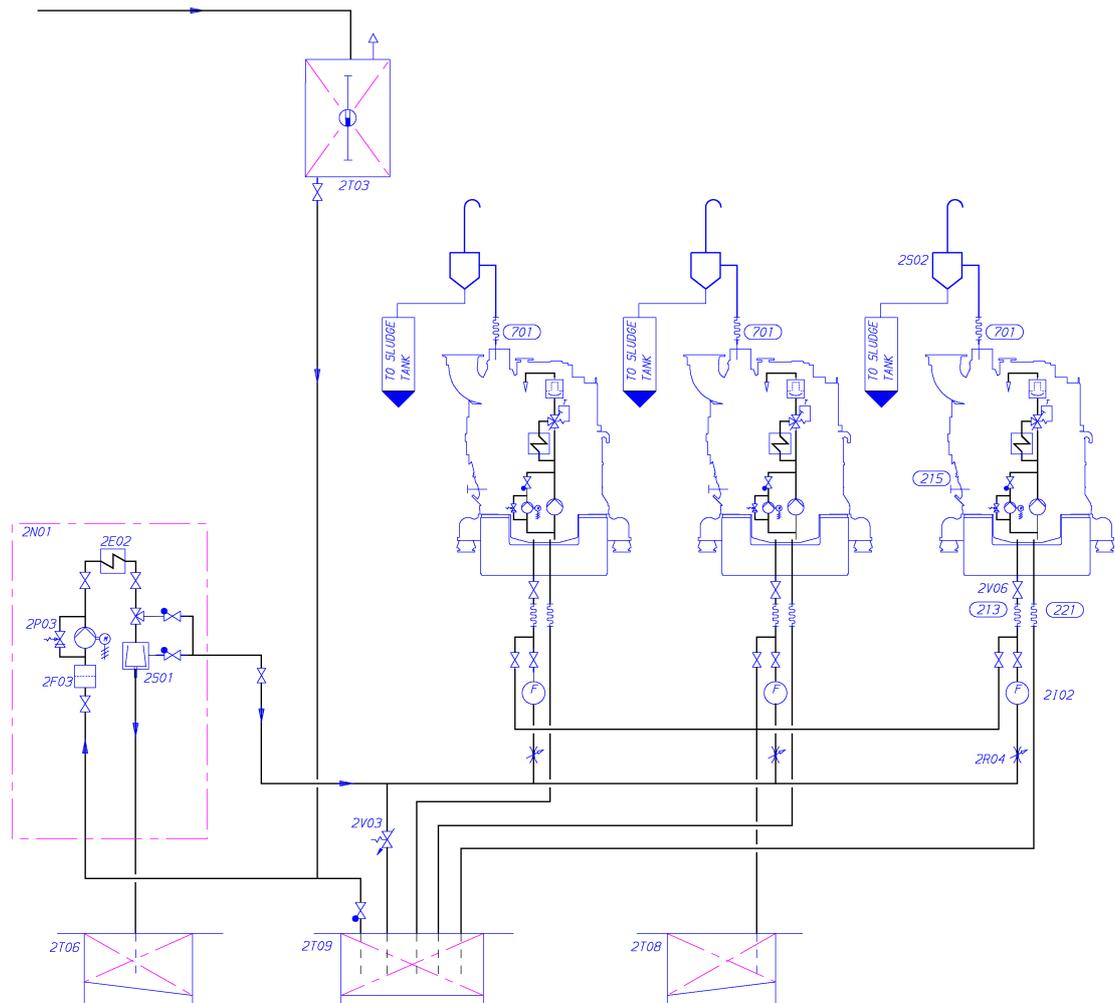
**Fig 6-5 External lubricating oil system WA20, overflow system (DAAE052029)**
