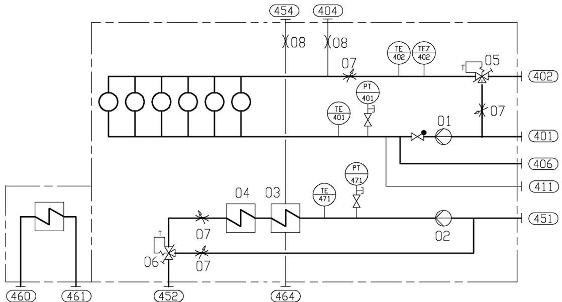
**Fig 8-1 Internal cooling water system, WA16, separate HT and LT (DAAF062367A)**
