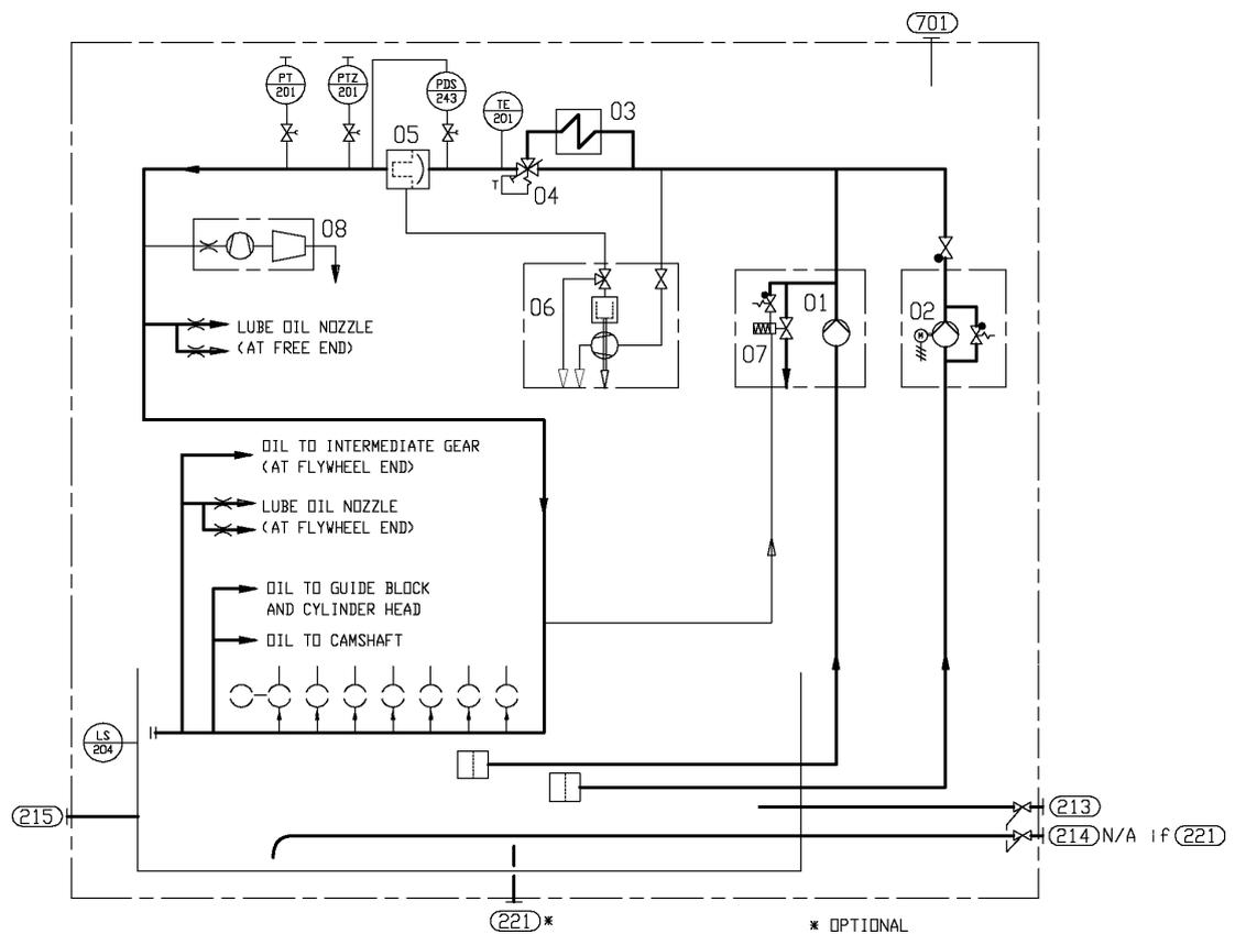
**Fig 6-1 Internal lubricating oil system, WA16 (DAAF062362A)**
