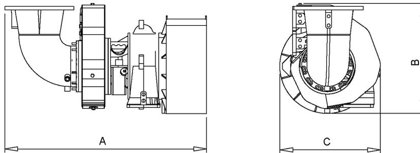
**Fig 18-3 Turbocharger**
