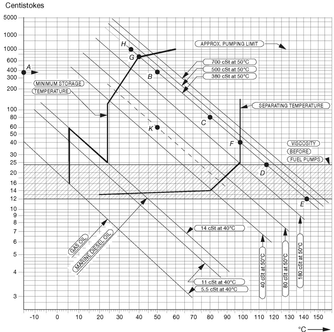
**Fig 5-4 Fuel oil viscosity-temperature diagram for determining the pre-heating temperatures of fuel oils (DAAE016379a)**
