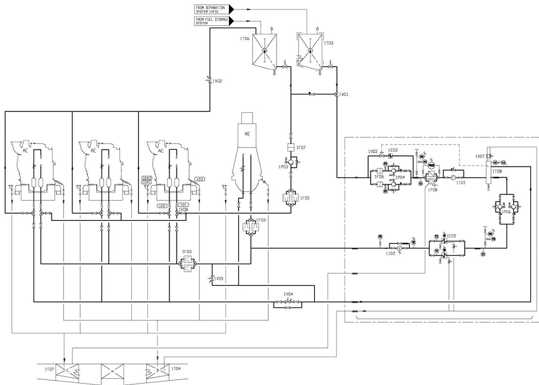
**Fig 5-8 Unifuel system, main and auxiliary engines (DAE006120f)**
