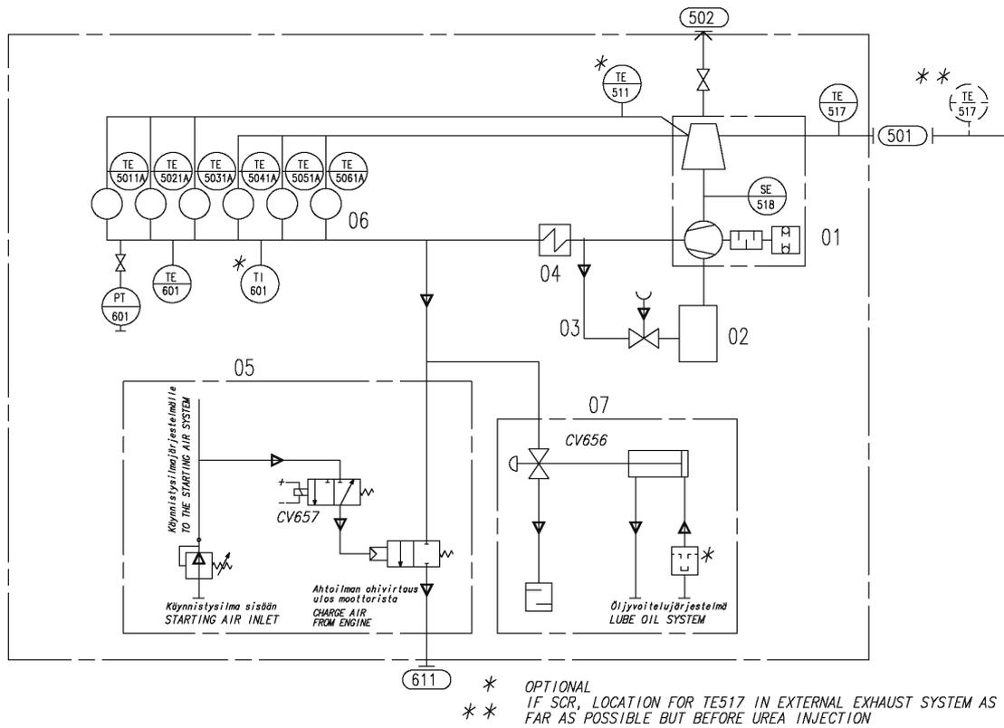
**Fig 10-2 Internal charge air and exhaust gas system, WA20 (DAAE010154D)**
