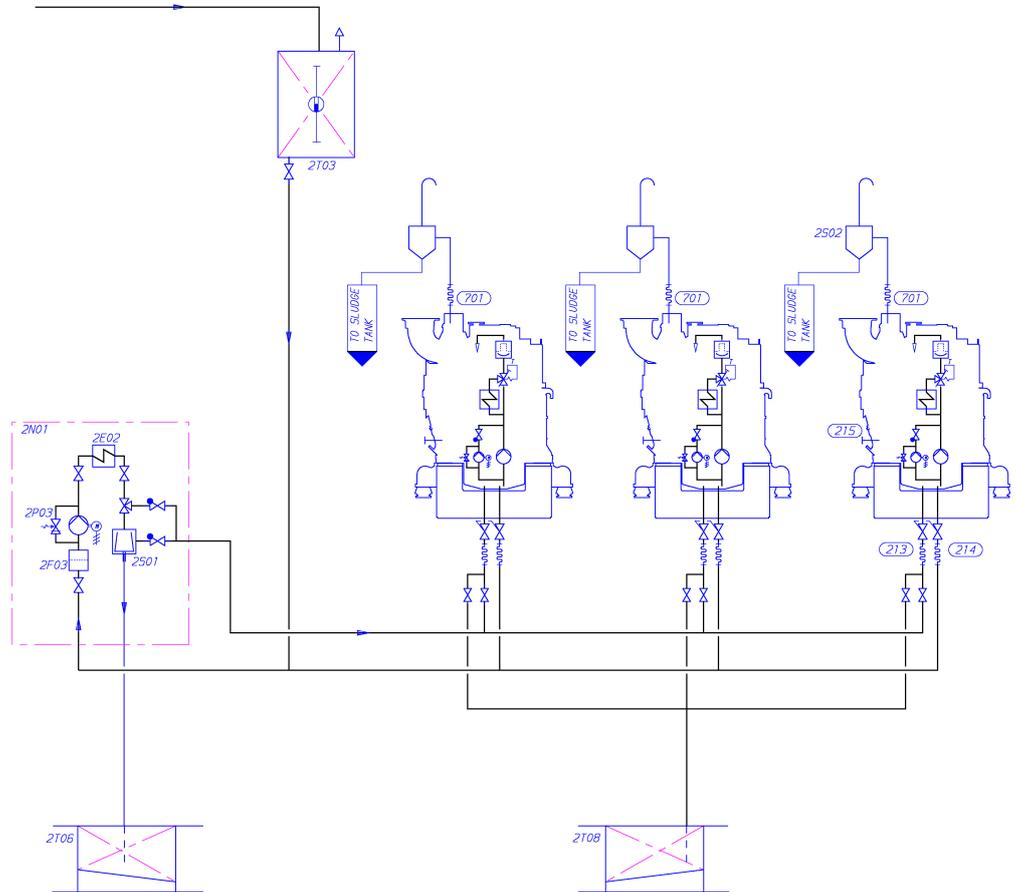
**Fig 6-6 External lubricating oil system, intermittent direct separation (DAAE052030a)**
