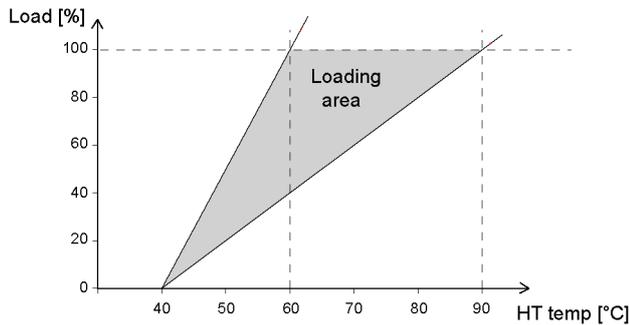
Fig 8-12 Load application on a cold generating set (20AP0703)
