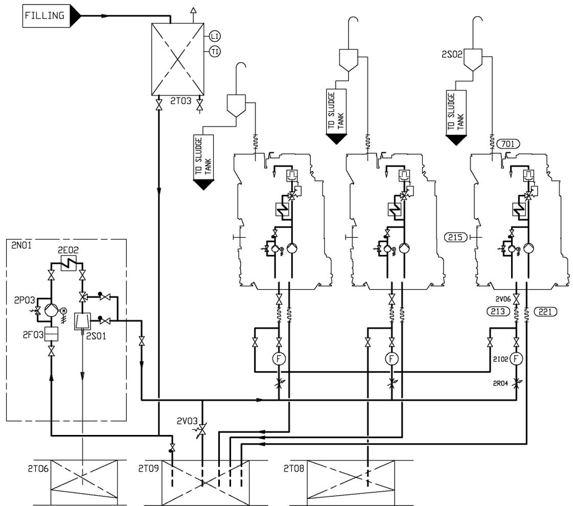
**Fig 6-4 External lubricating oil system for WA16, overflow system (DAAF062364A)**
