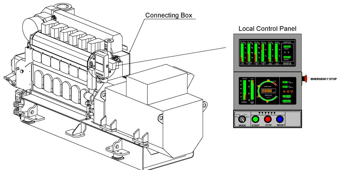
Fig 13-7 Connecting box and Local control panel
