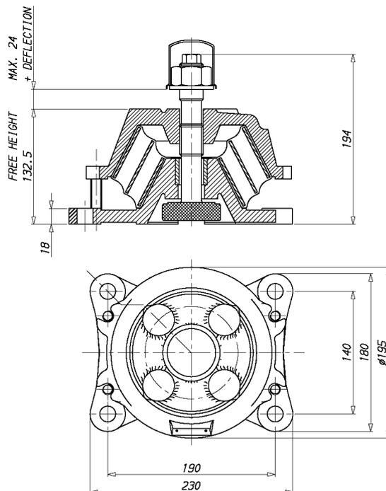
Fig 15-2 Rubber mounts W20
