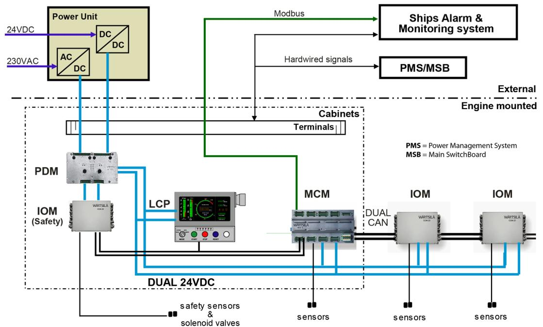
**Fig 13-1 Architecture of Engine Automation System**
