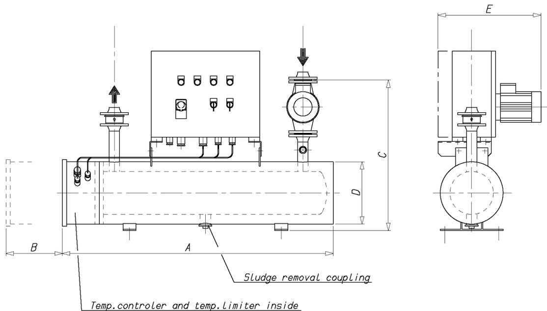
**Fig 8-13 Preheating unit, electric (3V60L0653a)**
