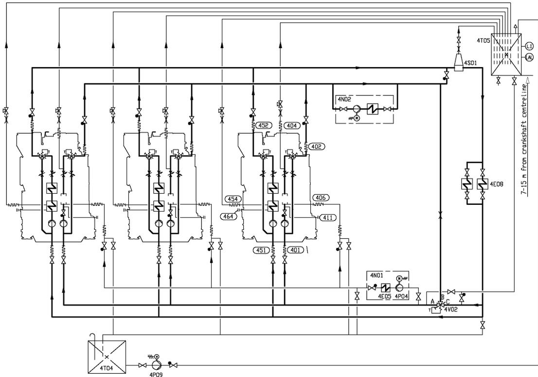
**Fig 8-6 Cooling water system, separate system for WA16 engines, with evaporator (DAAF062368A)**
