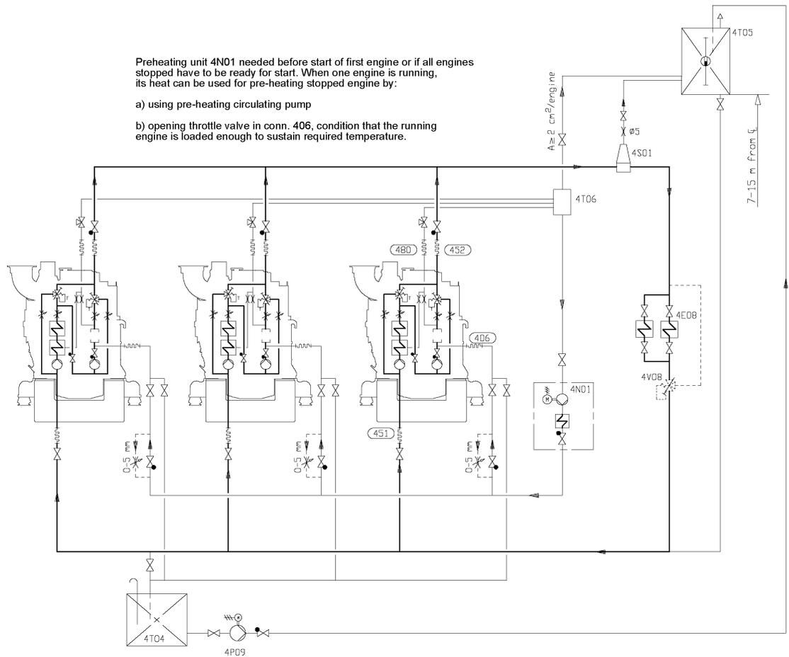
**Fig 8-5 Cooling water system, separate system for auxiliary engines, without heat recovery (DAAE028083b)**
