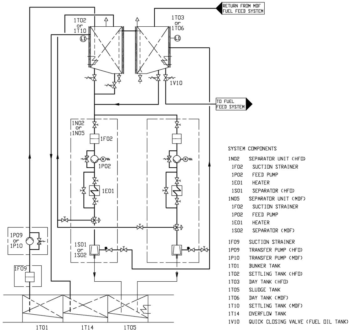
Fig 5-5 Fuel transfer and separating system (V76F6626F)
