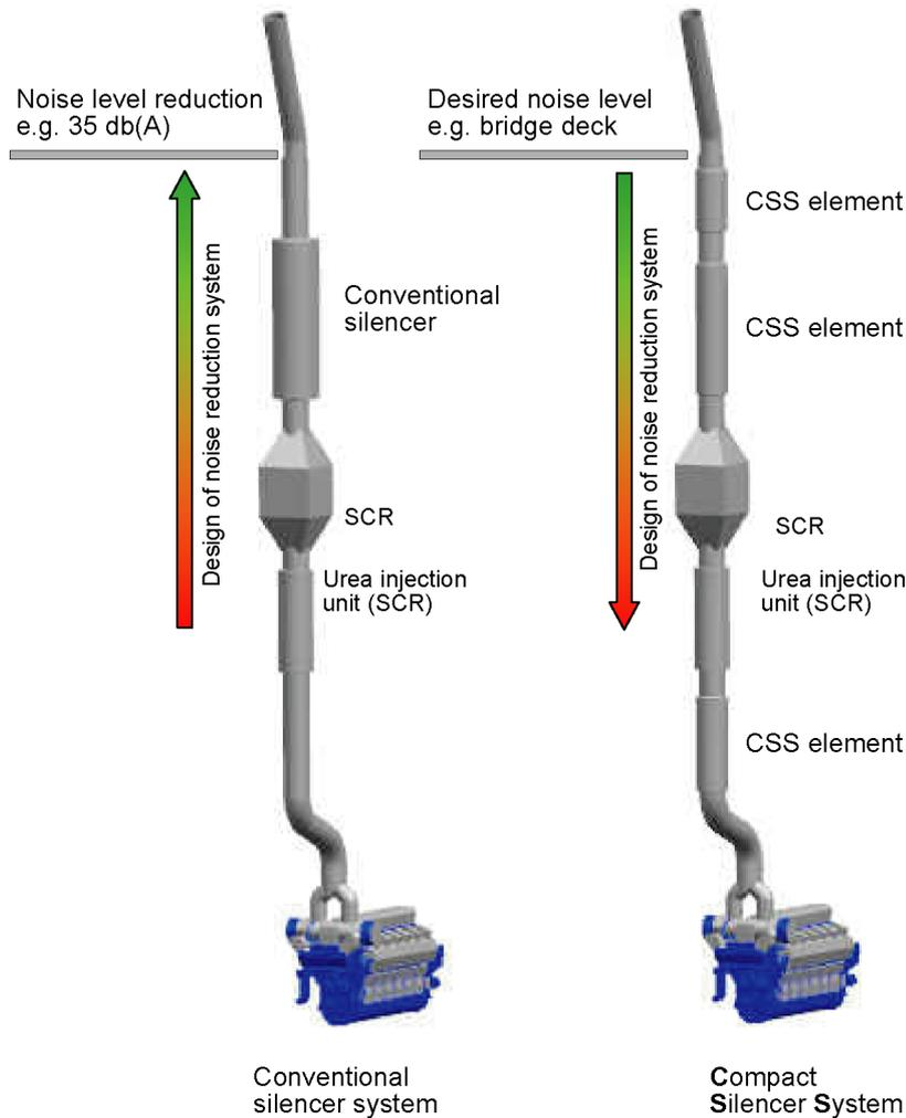
Fig 10-6 Silencer system comparison
