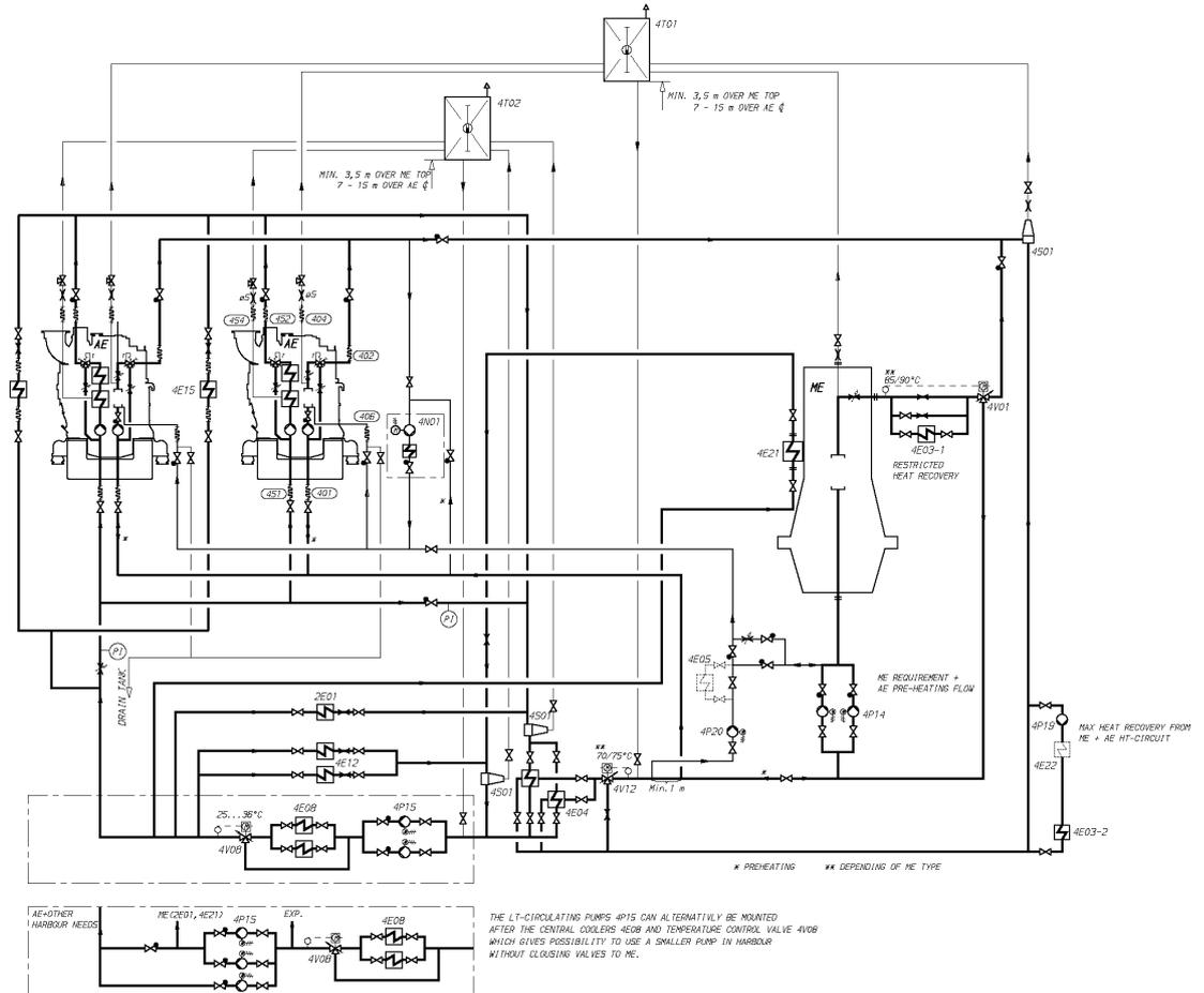
**Fig 8-9 Cooling water system, common for ME and AE, split LT- and HT-circuit, common heat recovery and preheating for ME and AE (DAAE030654A)**
