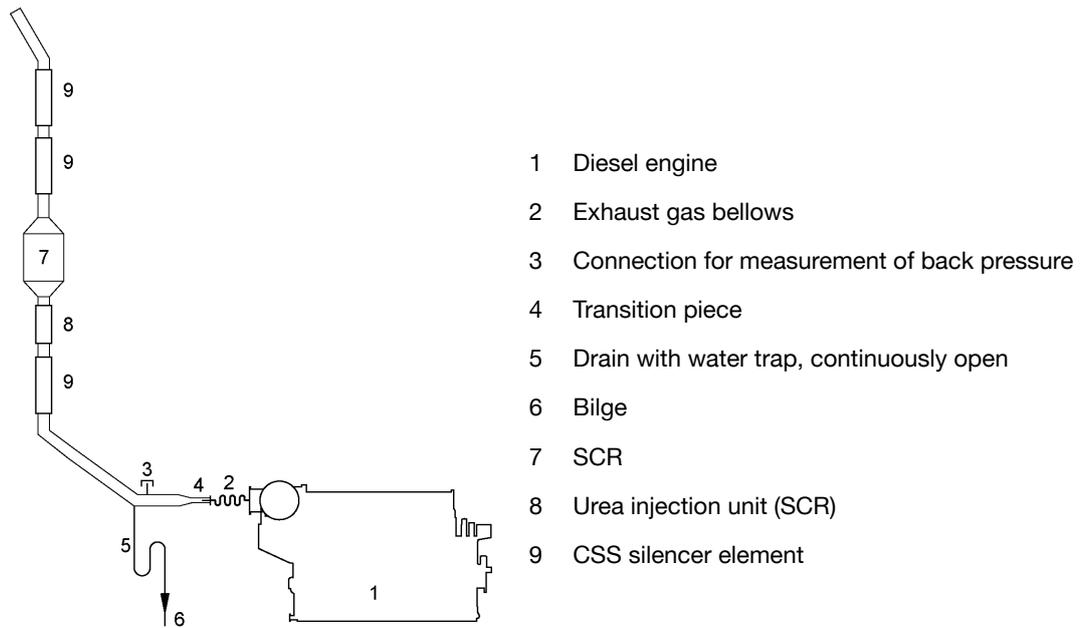
**Fig 10-4 External exhaust gas system**
