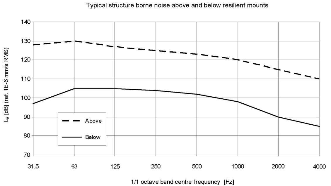
**Fig 16-1 Structure borne noise levels, WA20**
