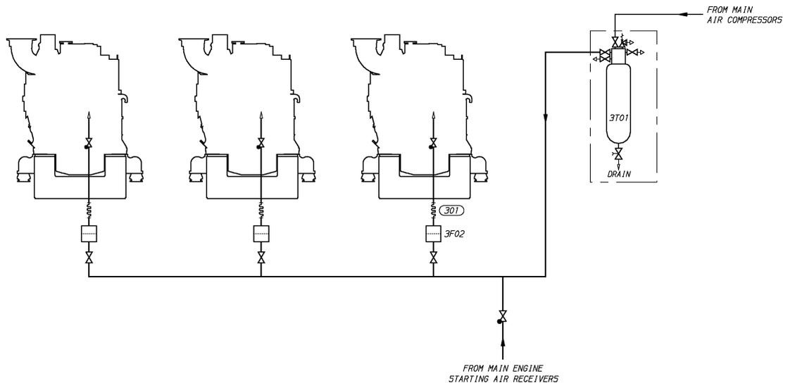
**Fig 7-3 Common external starting air system (DAAE007205d)**
