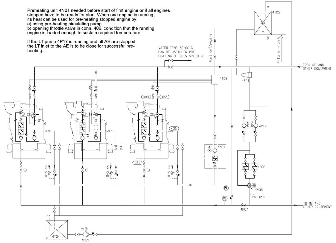
**Fig 8-11 Cooling water system, connected to a central LT system with circulating pump, without heat recovery (DAAE028652b)**
