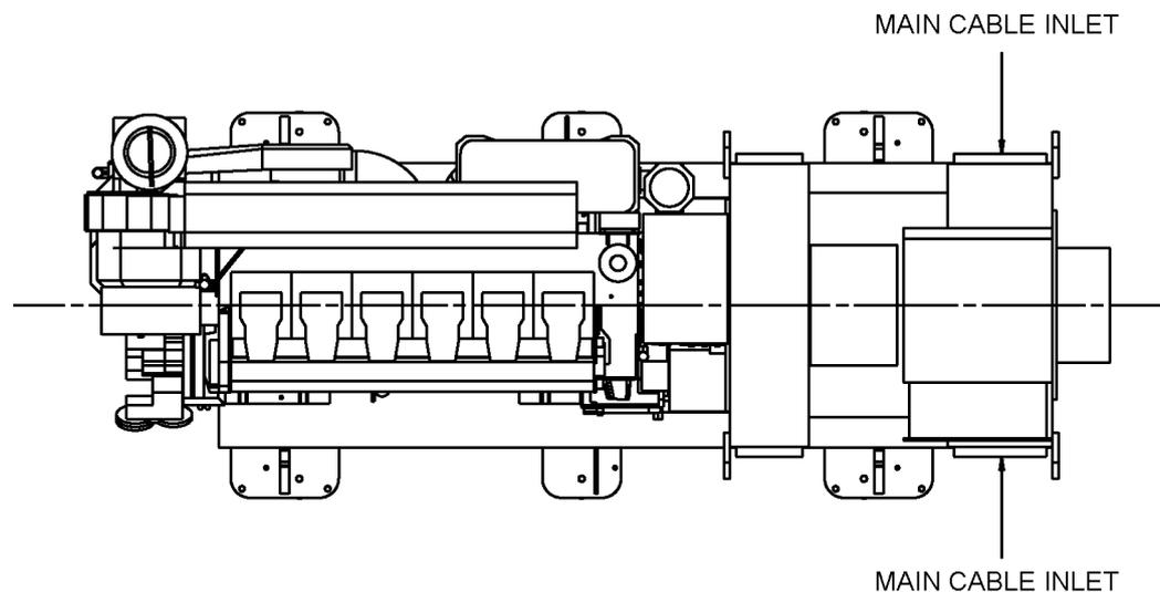
Fig 14-1 Connection of main cables (DAAE007153)
