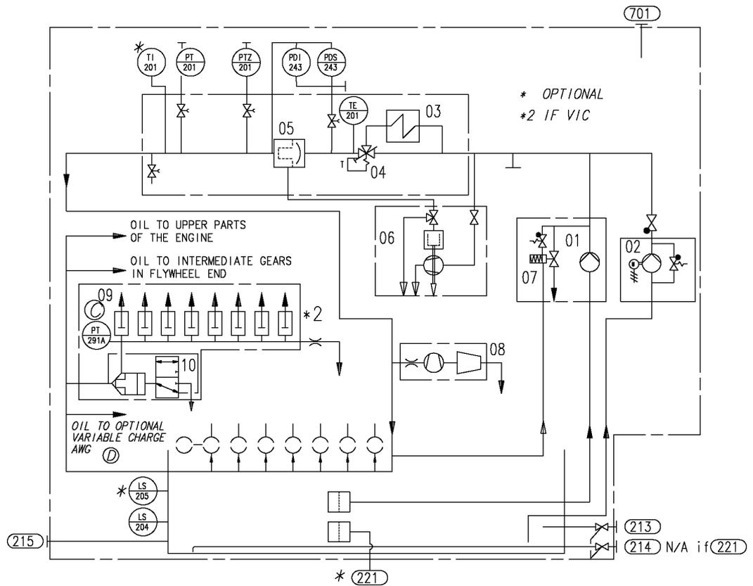
**Fig 6-2 Internal lubricating oil system, WA20 (DAAE010160D)**
