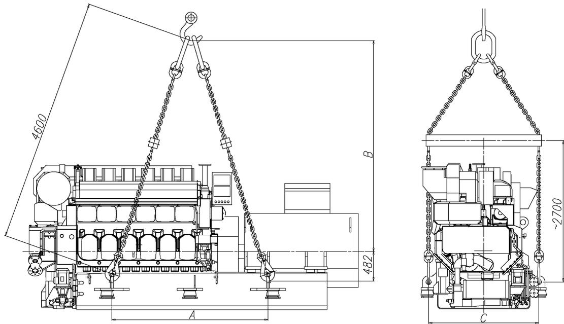
**Fig 18-2 Lifting of generating set (DAAE028691D)**
