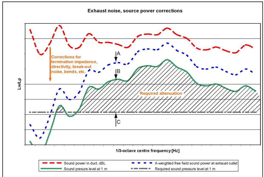
**Fig 10-5 Exhaust noise, source power corrections**
