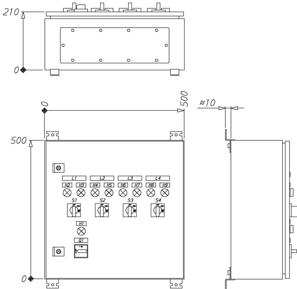
**Fig 13-8 Pre-lubricating pump starter (DAAE005967A)**
