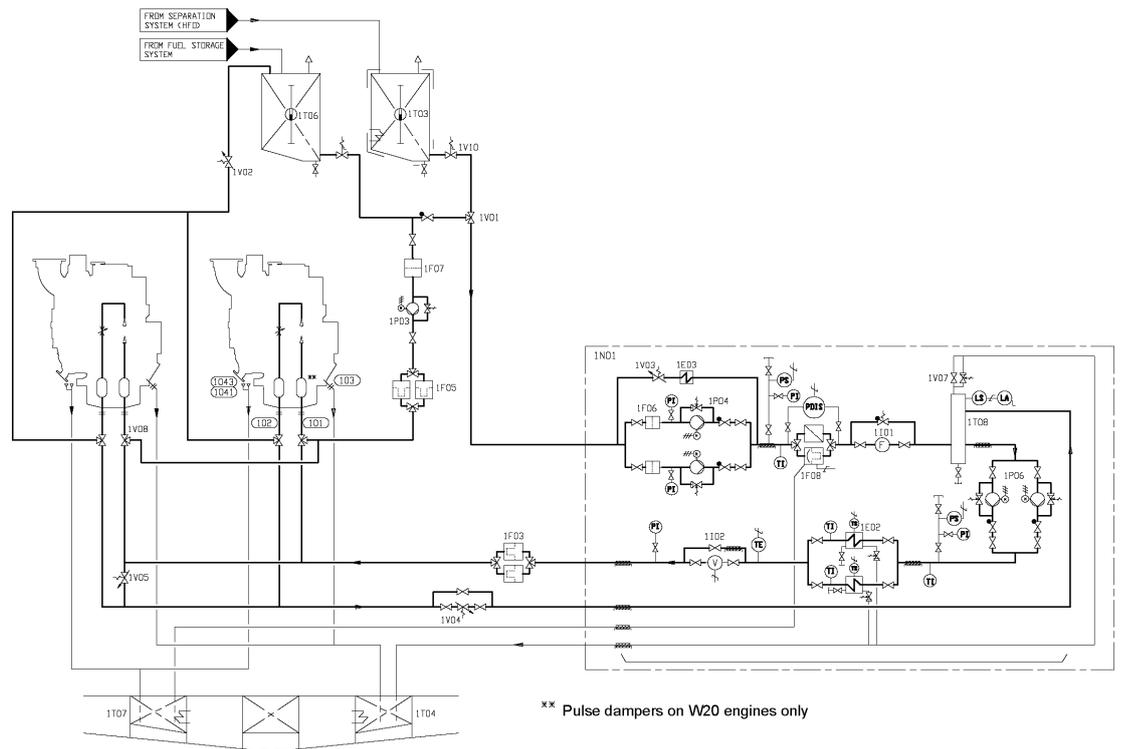
**Fig 5-7 External fuel system, HFO, two gensets (DAAE003609d)**
