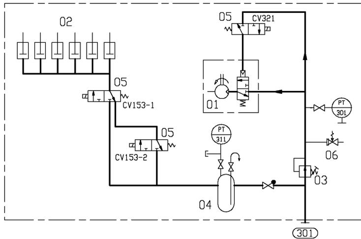
**Fig 7-1 Internal starting air system, WA16 (DAAF062365A)**
