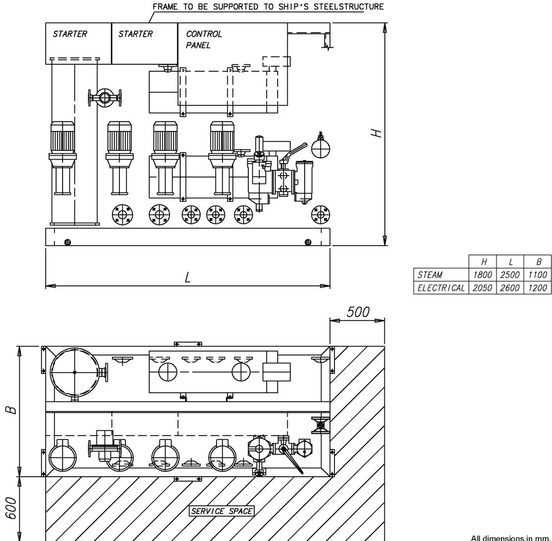
**Fig 5-9 Feeder/booster unit, example (DAAE006659)**
