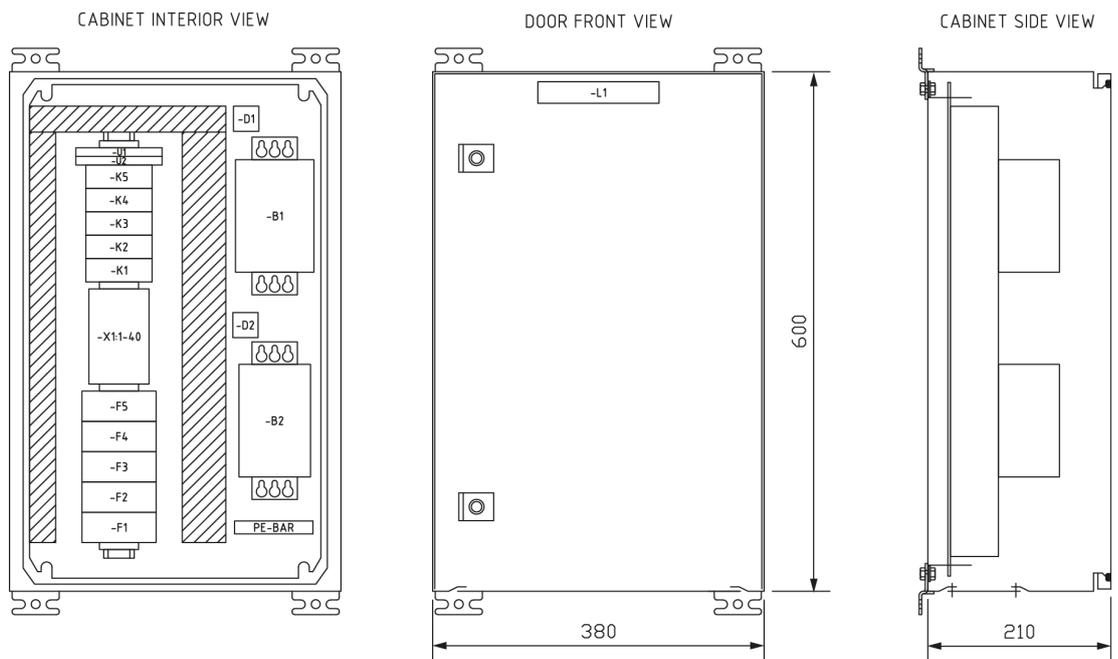
Fig 13-4 Standard power unit (DBAC145268)
