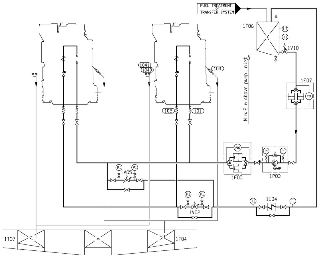
**Fig 5-3 External fuel oil system (MDF), WA16 (DAAF062360A)**
