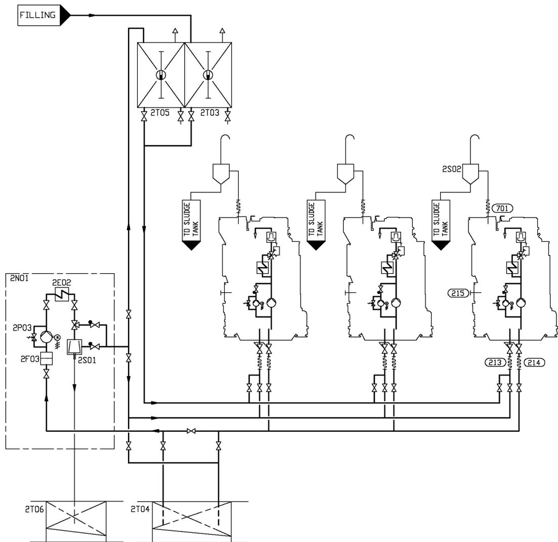
**Fig 6-3 External lubricating oil system, WA16 (DAAF062363)**
