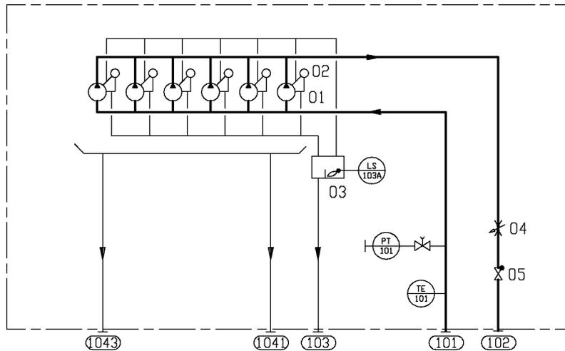
**Fig 5-1 Internal fuel oil system, WA16 (DAAF062359A)**
