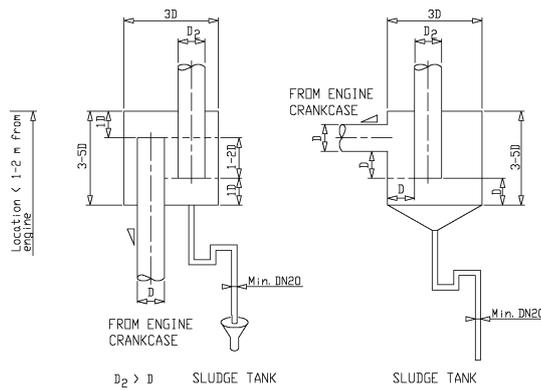
**Fig 6-7 Condensate trap (DAAE032780B)**
