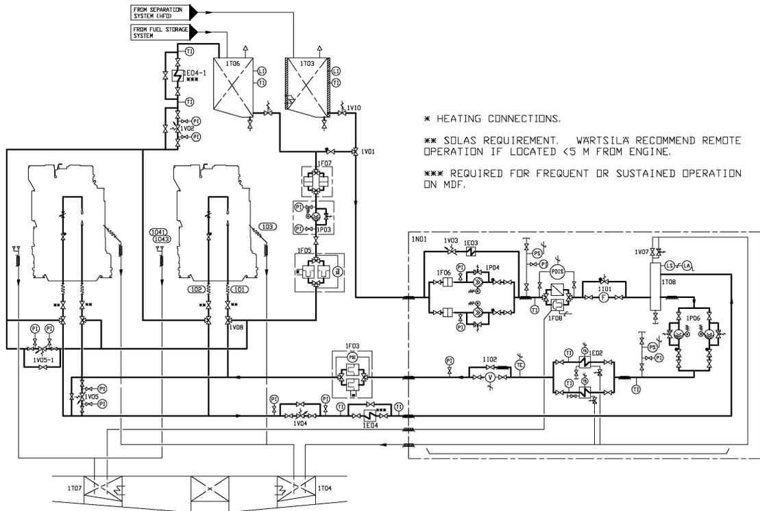
**Fig 5-6 External fuel system, WA16, two gensets (DAAF062361A)**
