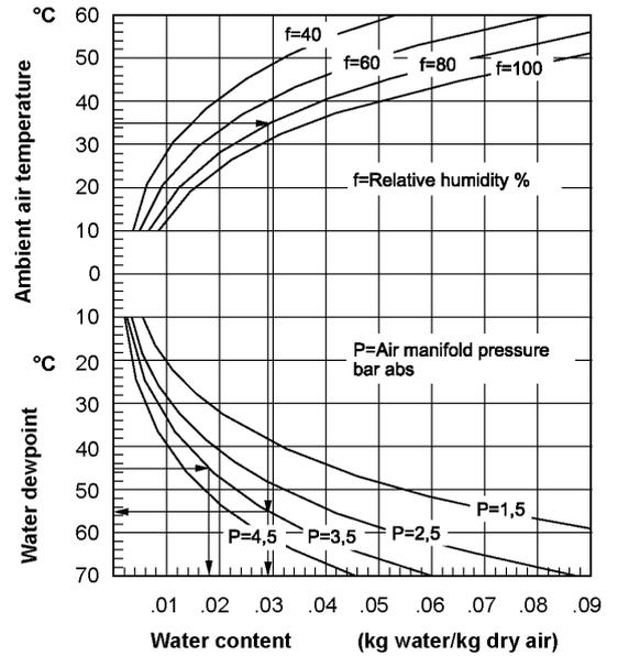
**Fig 9-1 Condensation in charge air coolers**
