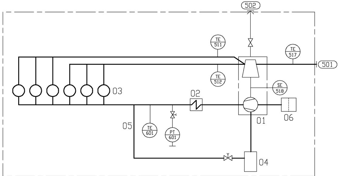
**Fig 10-1 Internal charge air and exhaust gas system, WA16 (DAAF062371A)**
