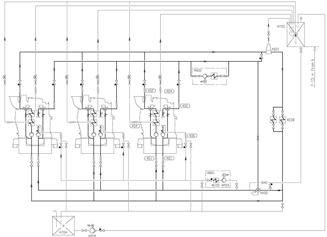
**Fig 8-7 Cooling water system, separate system for auxiliary engines, with evaporator (DAAF062369A)**
