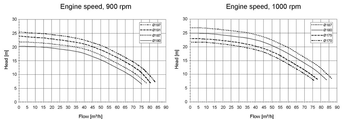
**Fig 8-4 W20 engine HT & LT-water pump curves**
