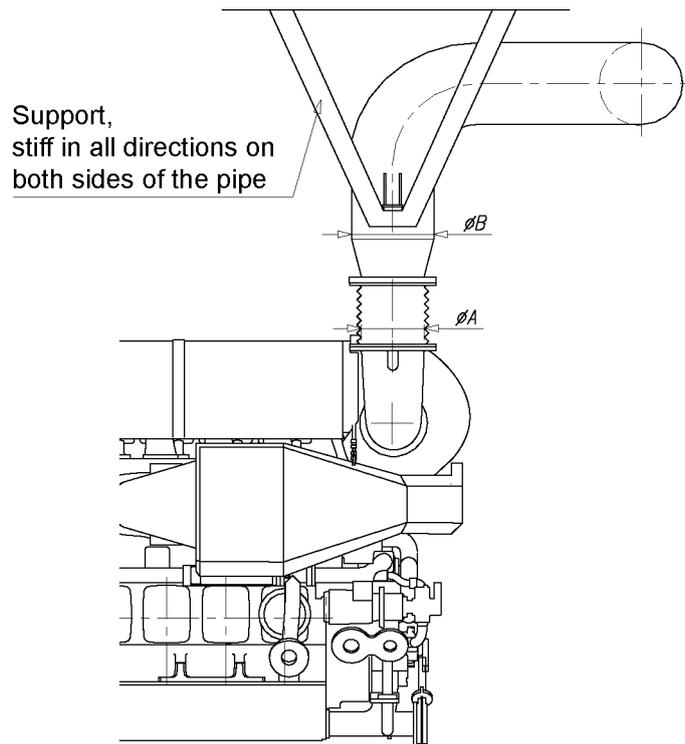
Fig 10-3 Exhaust pipe, diameters and support (DAAE011697A)
