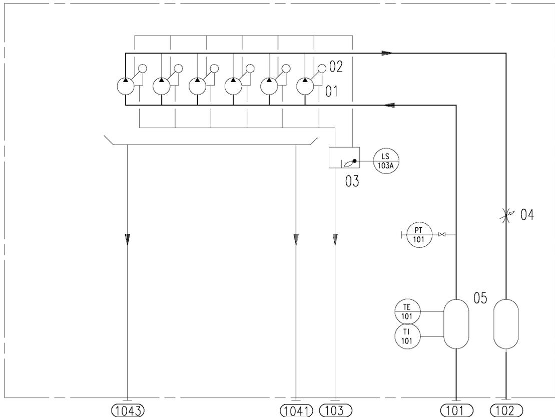
**Fig 5-2 Internal fuel oil system, WA20 (DAAE010153D)**
