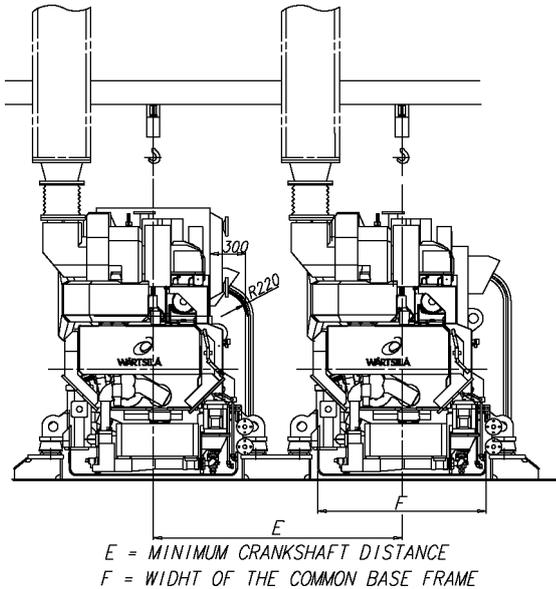
**Fig 17-1 Engine room arrangement, generating sets (DAAE028722D / DAAE048494 / DAAE041961)**
