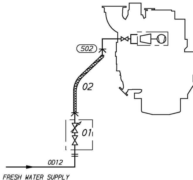
**Fig 11-1 Turbine cleaning system (DAAE003884)**
