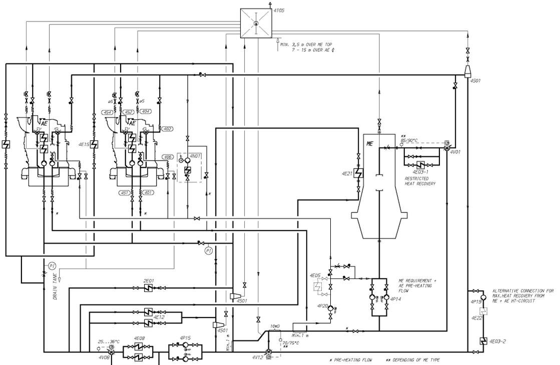
**Fig 8-10 Cooling water system, common for ME and AE, mixed LT- and HT-circuit, common heat recovery and preheating for ME and AE (DAAE030653A)**
