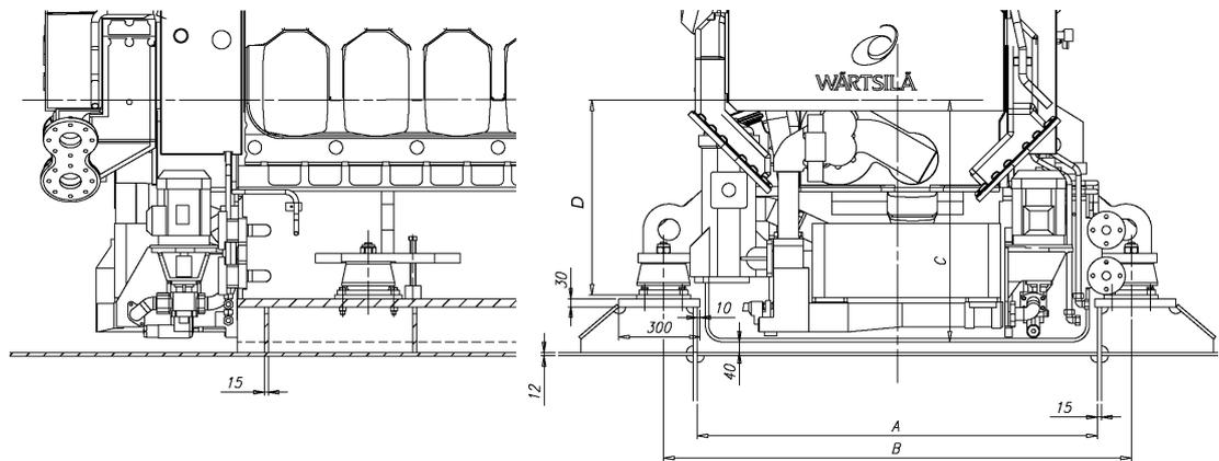
**Fig 15-1 Recommended design of the generating set seating (DAAE028099B / DAAE048324)**
