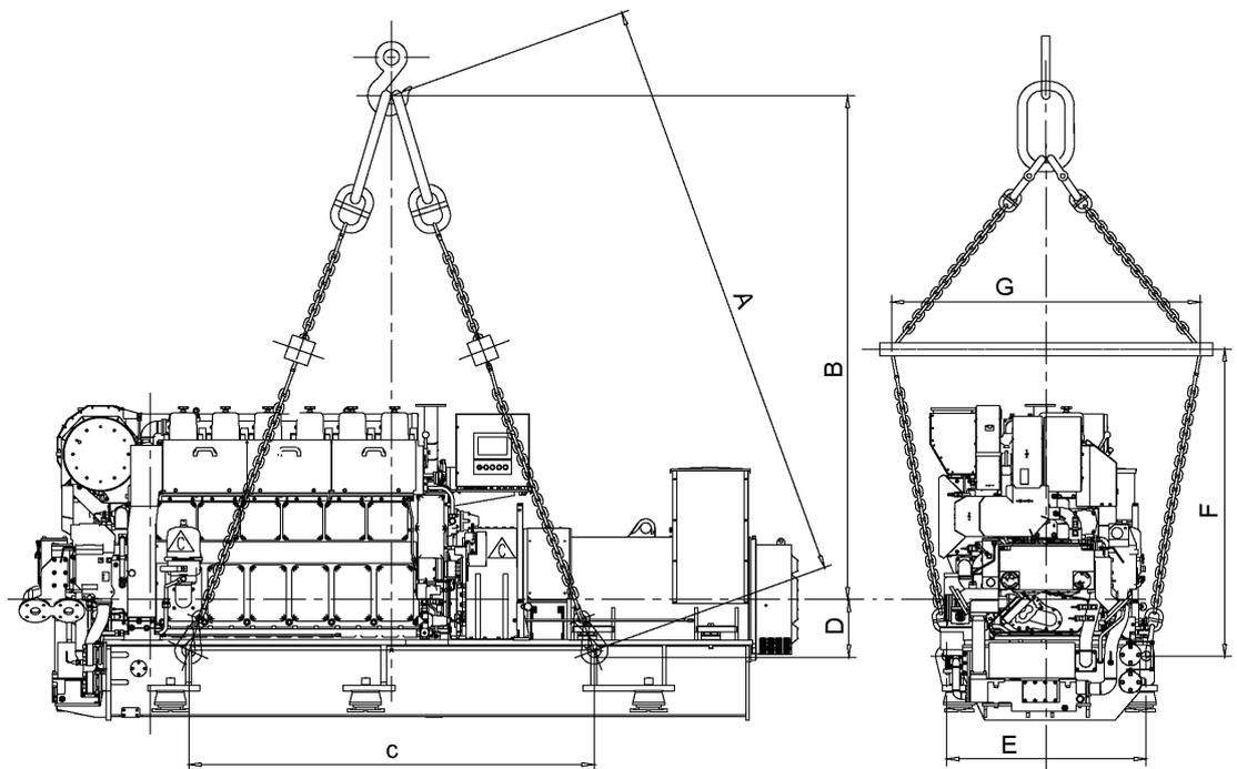
Fig 18-1 Lifting of generating set (DAAT003152C)
