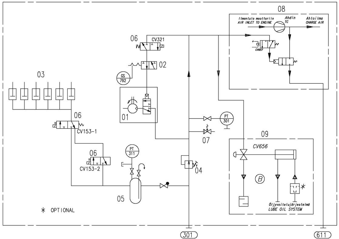
**Fig 7-2 Internal starting air system, WA20 (DAAE010155B)**
