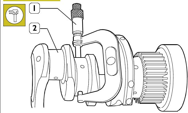
Grind journals and crankpins if seizing, scoring or excessive ovalisation are found. Before grinding the pins (2) measure them with a micrometer (1) to decide the final diameter to which the pins are to be ground.
