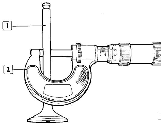
Check the valve stem (1) using a micrometer (2), it shall be  $6.970 \div 6.990$ .
