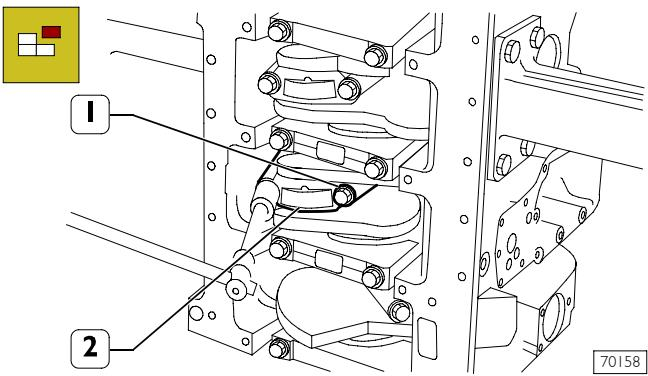
Loosen the fixing screws (1) and remove the rod caps (2). Withdraw the pistons including the connecting rods from the top of the engine block.
