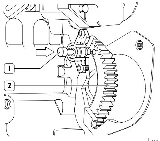
Turn the flywheel until, when pushing the pin 99360616 (1), it blocks the gear (2) obtaining the TDC of the 1° cylinder.
