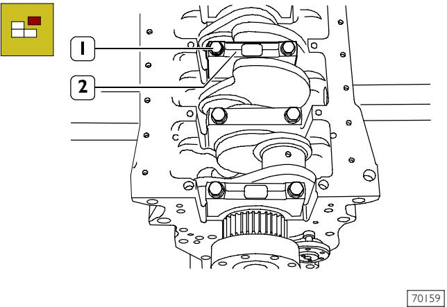
Remove the screws (1) and the main bearing caps (2).
