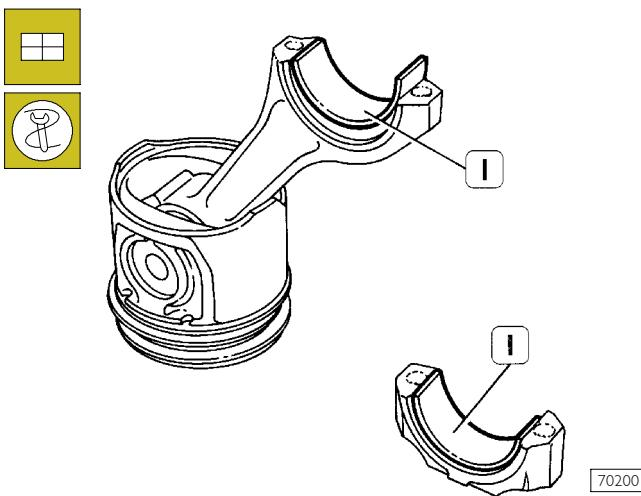
Fit half bearings (I) on connecting rod and cap.
