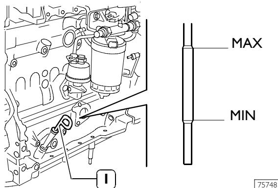
Draw off the rod from its slot and check that the level is within the etched tags of minimum and maximum level.
