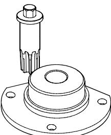
Tool for rotating/stopping the engine flywheel          |
