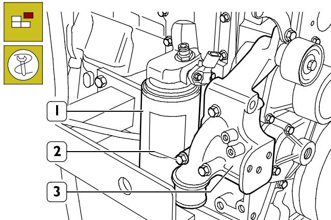
Remove the screws (2) and disconnect the alternator support (3).
