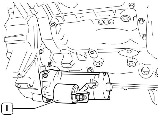
Starter is usually driven by starting unit placed on the vehicle dashboard and provides positive tension to the tele-switch assembled to the starter itself.
