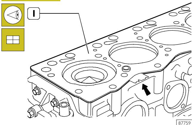
Check cleanliness of cylinder head and engine block coupling surface.
