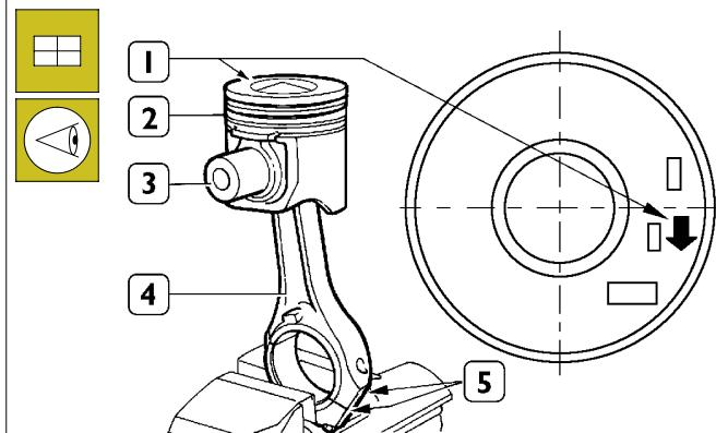
Connect piston (2) to connecting rod (4) with pin (3) so that the reference arrow (1) for fitting the piston (2) into the cylinder barrel and the numbers (5) marked on the connecting rod (5) are read as shown in the figure.
