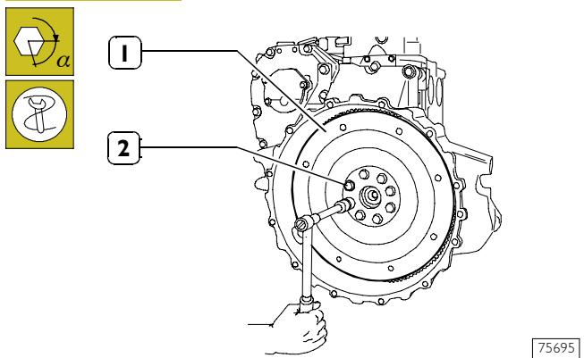
Tighten the engine flywheel (1) fixing screws (2) in two phases:
