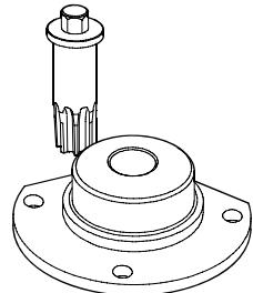
Tool for stopping the engine flywheel                   |
