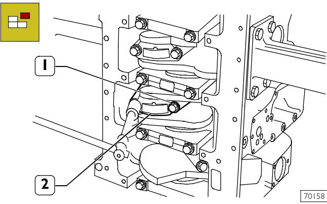
Remove the screws (1) fastening the connecting rod caps (2) and remove them.
