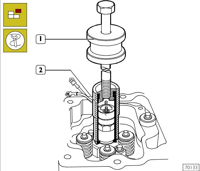
Remove injector fastening screws. Use tool 99342101 (1) to remove injectors (2) from the cylinder head.
