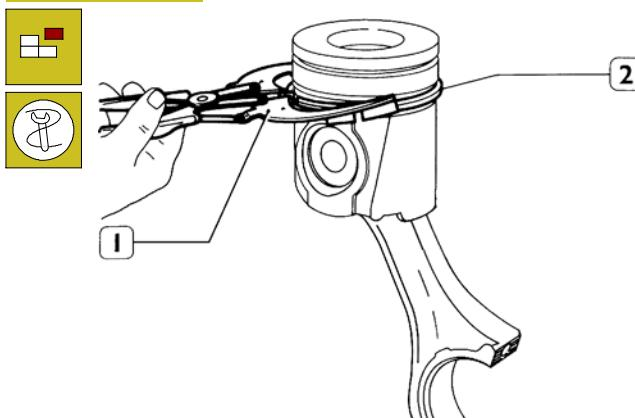
Remove split rings (2) from piston using pliers 99360183 (1).
