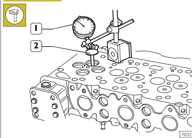
Use a magnetic base dial gauge (1) set as shown in the figure, the assembling clearance shall be  $0.052 \div 0.092$  mm.
