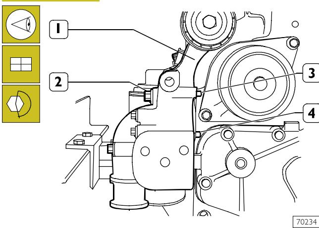
Position the alternator support (1) so that pins (3 and 4) are set against the engine block.
