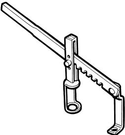
Tool for removing/refitting engine valves               |
