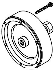
Tool to remove output shaft rear gasket                                    |
