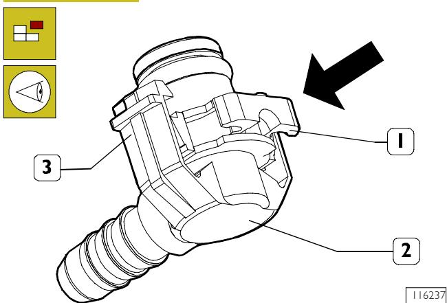
To disconnect the low pressure fuel pipe from the relevant connecting joint, you need to hold the clasp (1) pressed, and release the quick fitting joint (2).
