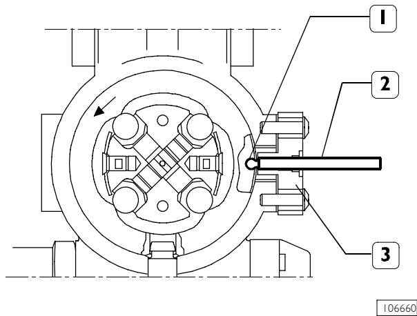
1. Slot on the hub of the hydraulic rotor -
