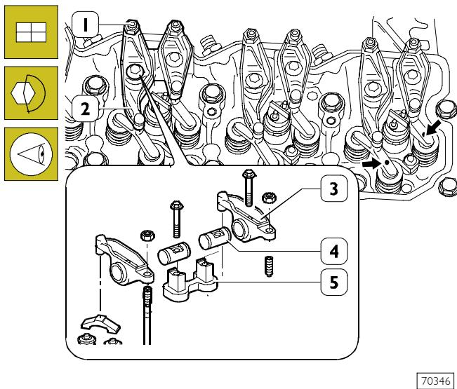
Check that tappet adjusters (1) are loose to prevent their balking on the rods (2, Figure 90) when refitting the rocker assembly.
