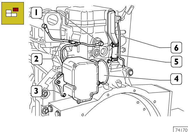
Disconnect the pipeline (2) from the fuel recover pressure-limiter, working on the connections as described in Figure 3.
