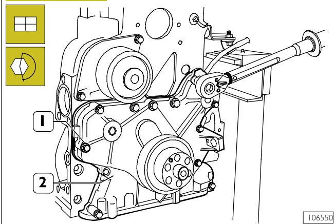
Clean accurately the front cover (2) surface and refit it. Tighten the screws (1) to the specified torque.
