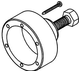
Tool to remove output shaft front gasket                                   |
