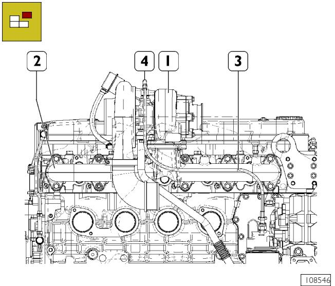
Disconnect the oil pipeline (3) from the supports of the heat exchanger / oil filter and from the pipe fitting (4) to the turbine.
