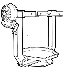
Revolving stand for overhauling units (700 daN/m capacity, 120 daN/m torque) |
