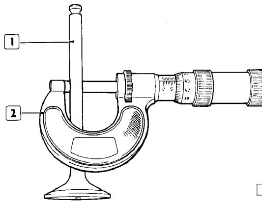
Check the valve stem (1) using a micrometer (2), it shall be 7.943 to 7.963.
