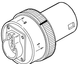
Adaptors for 38 to 30 pin connectors (component of 99368554)               |
