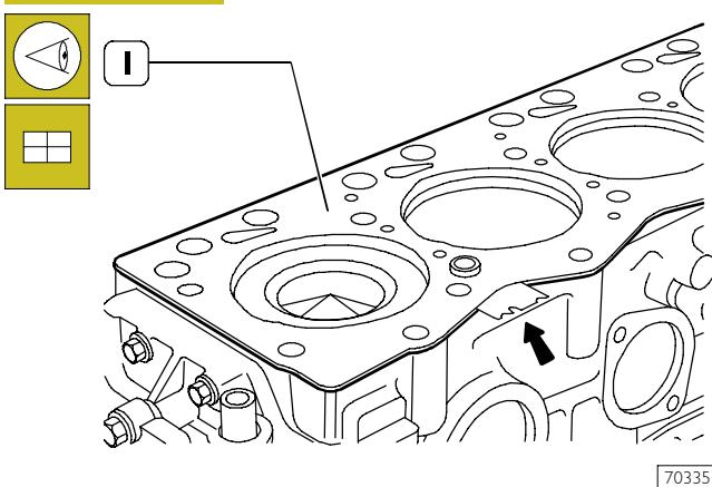
Check cleanliness of cylinder head and engine block coupling surface.
