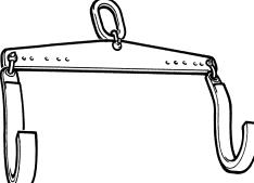
Tool for lifting the output shaft                                        |
