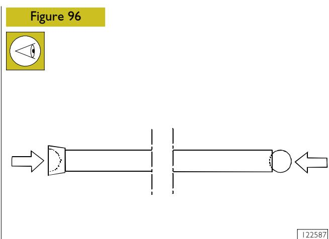
Before executing assembly, check the Rocker Arm driving rods: these shall not be deformed; the spherical ends in contact with the Rocker Arm adjustment screw and with the tappet (arrows) shall not present evidence of seizure or wear: in case of detection proceed replacing them.
