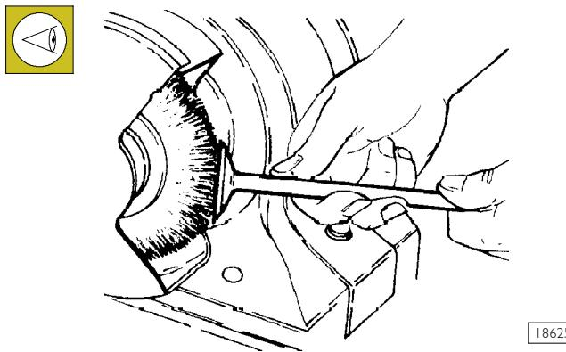
Remove carbon deposits from valves using the proper metal brush.
