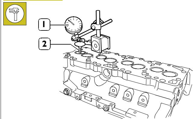
Use a magnetic base dial gauge (1) set as shown in the figure, the assembling clearance shall be  $0.056 \pm 0.096$  mm.
