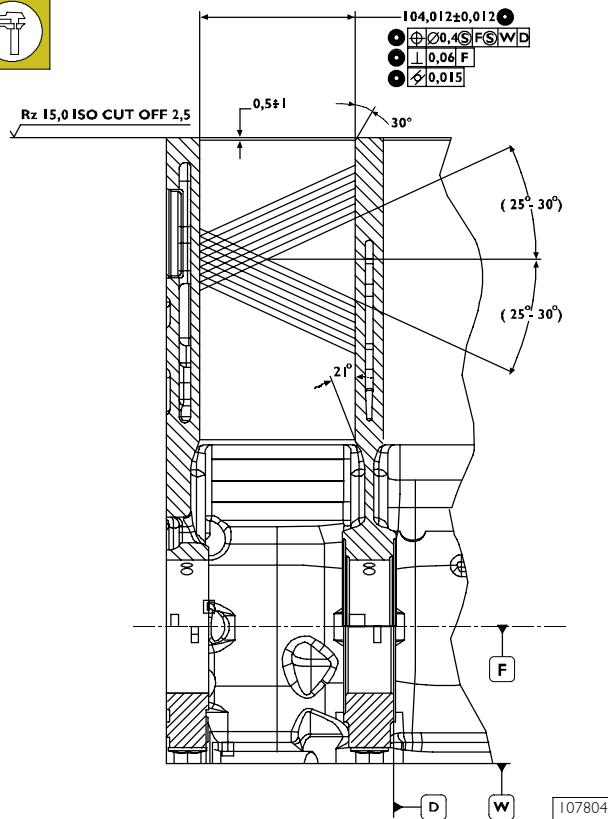
**NOTE** In case of regrinding, all barrels shall have the same oversize (0.4 mm).
