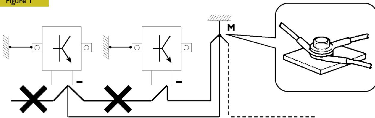
I. NEGATIVE CABLES "STAR" CONNECTION TO SYSTEM BONDING M
