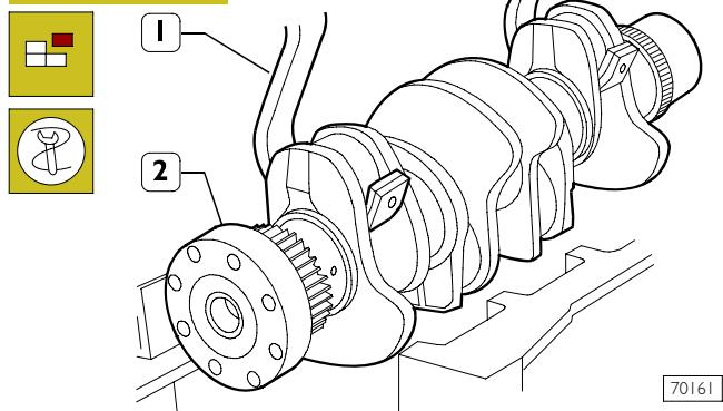
Use tool 99360500 (1) and hoist to remove the crankshaft (2) from the block.
