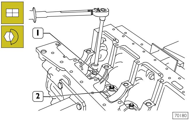
Fit nozzles (2) and tighten the fastening screws (1) to the specified torque.
