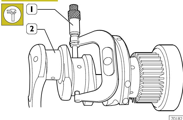
Grind journals and crankpins if seizing, scoring or excessive ovalisation are found. Before grinding the pins (2) measure them with a micrometer (1) to decide the final diameter to which the pins are to be ground.
