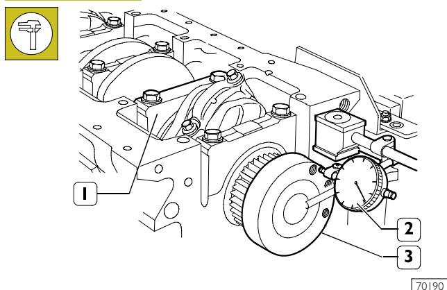
This check is performed by setting a magnetic-base dial gauge (2) on the crankshaft (3) as shown in the figure, standard value is 0.068 to 0.41.
