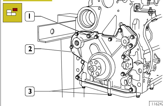
Remove the screws (1 and 3) and take out the front cover (2).
