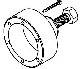
Tool to remove output shaft front gasket                                    |
