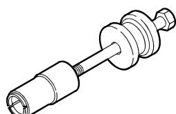
Tool to remove injectors
