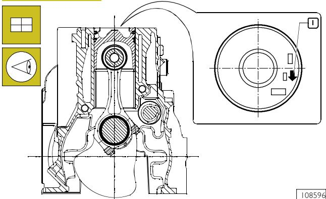
**DIAGRAM FOR CONNECTING ROD-PISTON ASSEMBLY FITTING INTO BARREL**
