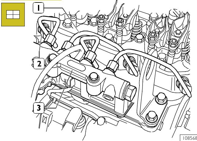
Connect new fuel pipes (1) to rail (3) and injector manifolds (2).
