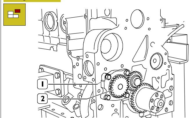
Remove the screws (1) and disconnect the oil pump (2).
