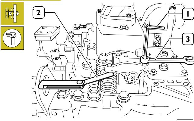
Adjust the play between the rocker arms and valves using a hex key (1), polygonal key (3) and feeler gauge (2).
