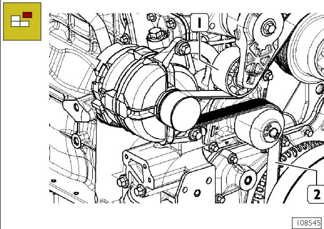
Release on the drive belt tensioner (1) and extract the belt (2) from the belt pulleys from the water pump ones and from the belt rebound pulleys;
