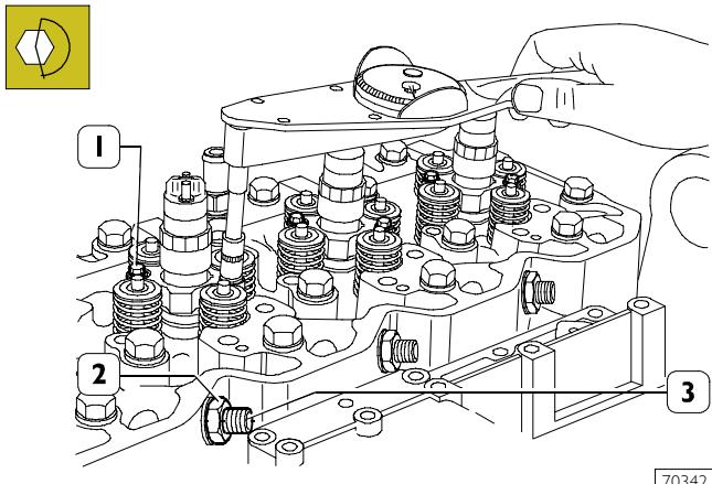
Use the torque wrench to tighten gradually and alternately the injector fastening screws (1) to  $8.5 \pm 0.8$  Nm torque.
