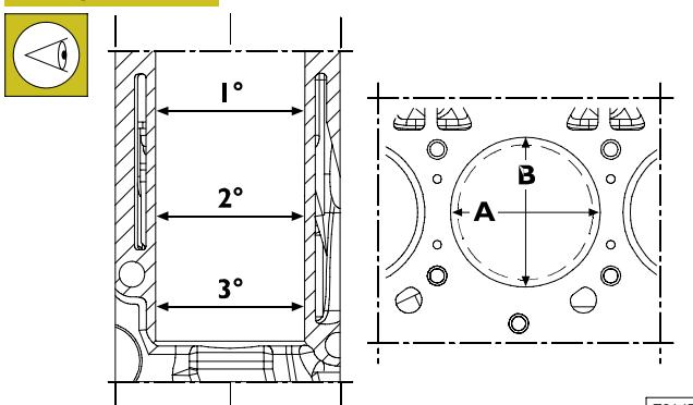
Measurements shall be performed on each cylinder, at three different heights in the barrel and on two planes perpendicular with each other: one parallel to the longitudinal axis of the engine (A), and the other perpendicular (B). Maximum wear is usually found on plane (B) in correspondence with the first measurement.
