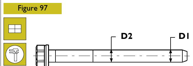
Insert the tappet driving rods and the Rocker Arm unit. Before using the fixing screws again, measure them twice as indicated in the picture, checking D1 and D2 diameters:
