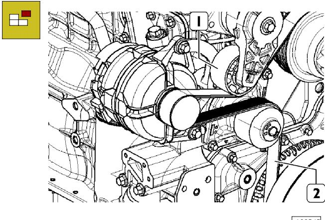
Release on the drive belt tensioner (1) and extract the belt (2) from the belt pulleys from the water pump ones and from the belt rebound pulleys;
