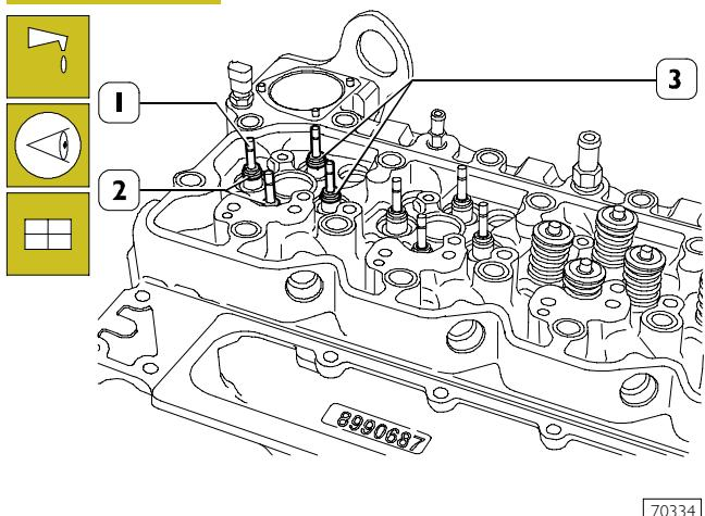
Lubricate the valve stems (1) and fit them into the relevant valve guides according to the position marked at removal.
