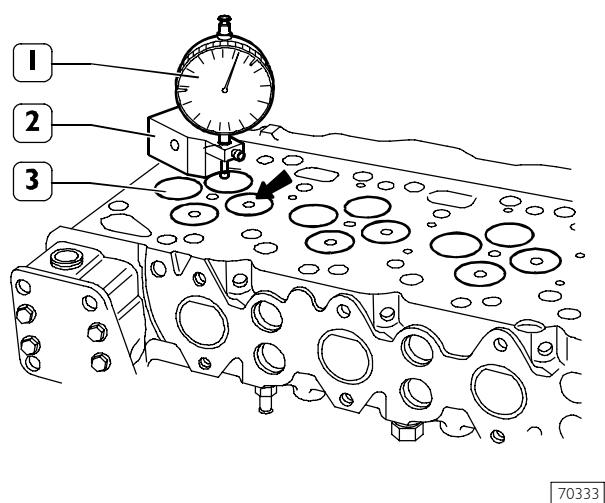
After regrinding, check that valve (3) sinking value is the specified one by using the base 99370415 (2) and the dial gauge 99395603 (1).
