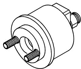
Tool for fitting output shaft front gasket
