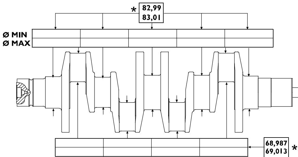
FILL THIS TABLE WITH OUTPUT SHAFT JOURNAL AND CRANKPIN MEASURED VALUES
