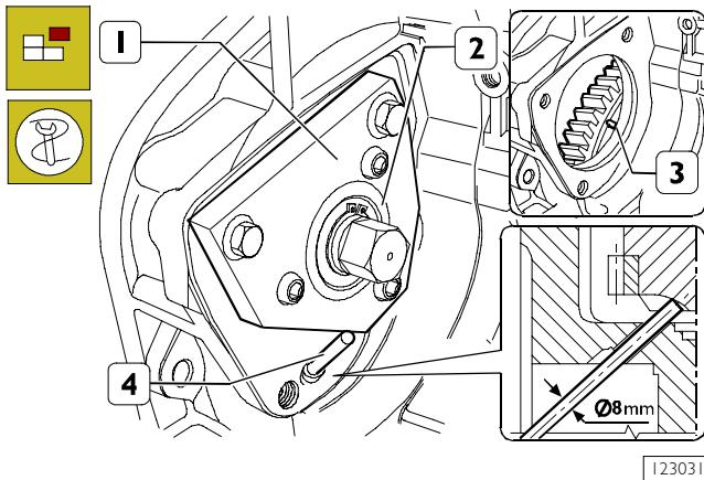
Disassemble the starter from the flywheel box and use tool 99360339 (1) to rotate the flywheel.
