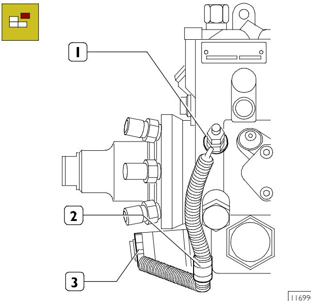
Disconnect the linkage connector from the temperature sensor on the motor, and then remove the fixing nut of the socket clamp (2) and the nut (1) of the cable group end, so to release the electrical lead assembly of the solenoid valve throttle.
