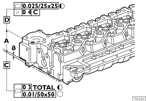
The rated thickness A for the cylinder head is  $105 \pm 0.25$  mm, max. metal removal shall not exceed thickness B by 1 mm.
