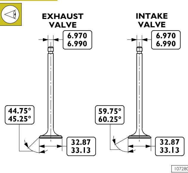
INTAKE AND EXHAUST VALVE MAIN DATA
