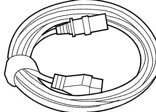
Adaptor (5m) for tester PT01 connection to 30 pin test socket (component of 99368554)                |
