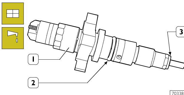
Fit a new sealing ring (2) lubricated with petroleum jelly and a new sealing washer (3) on injector (1).
