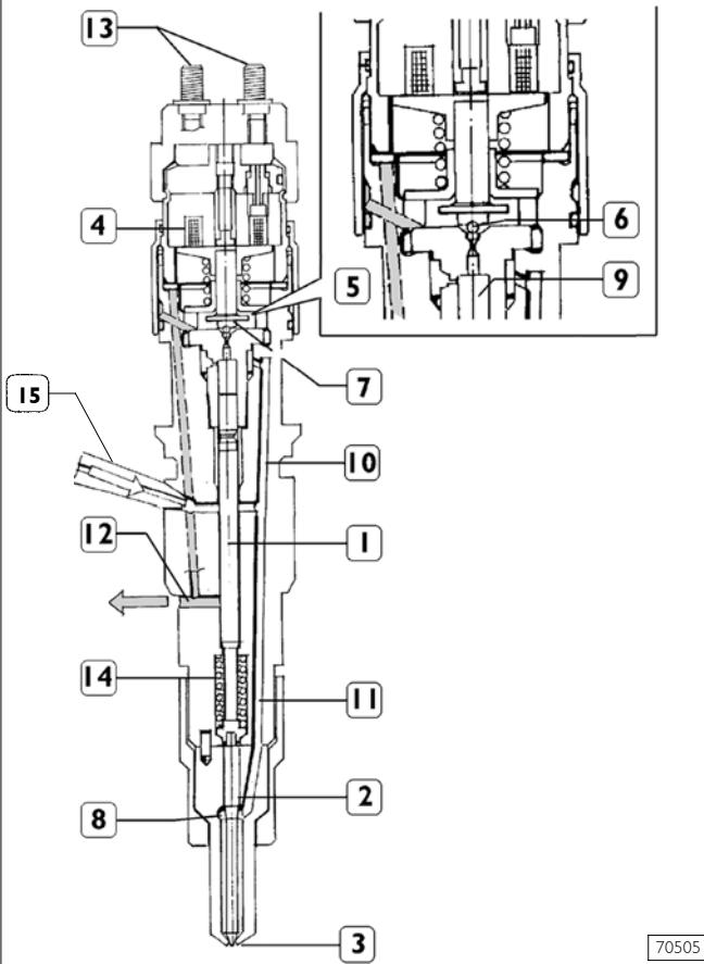
1. Pressure rod – 2. Plunger – 3. Nozzle – 4. Coil – 5. Pilot valve – 6. Ball shutter – 7. Control area – 8. Pressure chamber – 9. Control volume – 10. Control duct – 11. Supply duct – 12. Control fuel outlet – 13. Electric connection – 14. Spring – 15. High-pressure fuel inlet.
