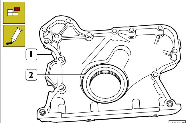
Remove the sealing ring (2) from the front cover (1), clean accurately the coupling surfaces and smear them with LOCTITE 5205.
