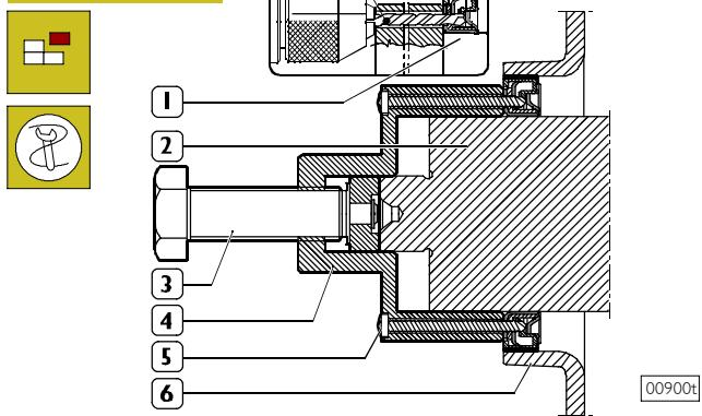
Remove the ring sealing the engine's driving shaft from the front cover. Use the tool 99340055 (4) to operate on the front bar hold of the driving shaft. Through the steering holes of the tool, perforate the inside holding ring (1) with a straight way drill (diam. 3,5mm) for the depth of 5mm. Fix the tool to the ring tightening the 6 screws provided with the equipment. Then proceed removing the ring (2) by tightening the screw (3).
