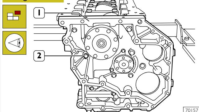
Remove the screws (2) and disconnect the timing gear case (1).
