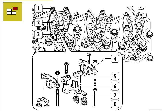
Loosen tappet adjustment fastening nuts (1) and unscrew the adjusters.
