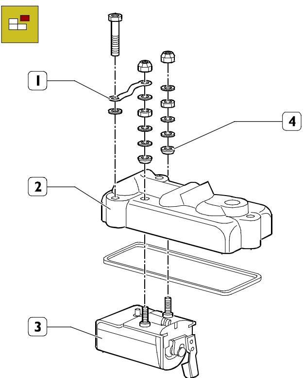
Remove the electro-valve (3) from the cover (2).
