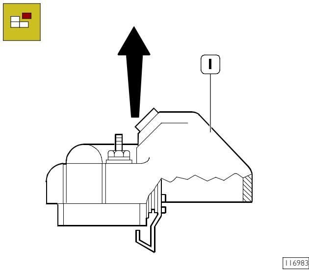
Remove the entire cover of the electro-valve (1), pulling it upwards perpendicularly to the injection pump.
