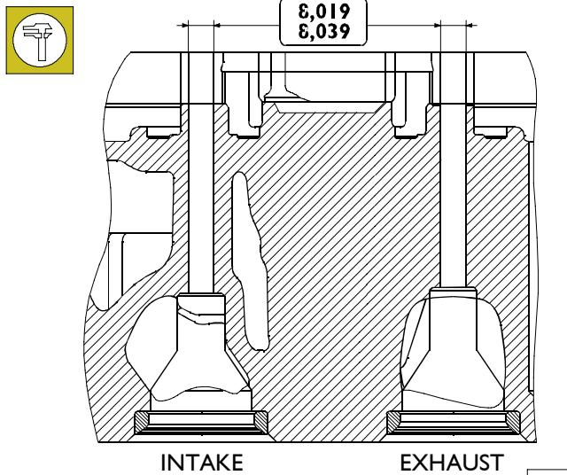
Use a bore dial gauge to measure the inside diameter of the valve guides, the read value shall comply with the value shown in the figure.
