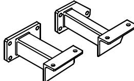
Brackets for fastening engine to revolving stand 99322205               |
