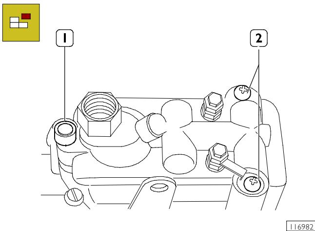
To replace the electro-valve remove the cover of the injection pump loosening and removing the three fixing screws (1 and 2) of the cover and the relative washers.
