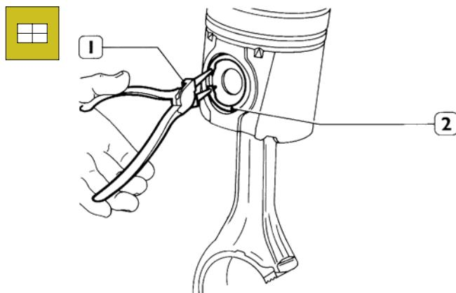
Position the piston on the connecting rod according to the diagram shown in the figure, fit the pin and stop it by the split rings (2).
