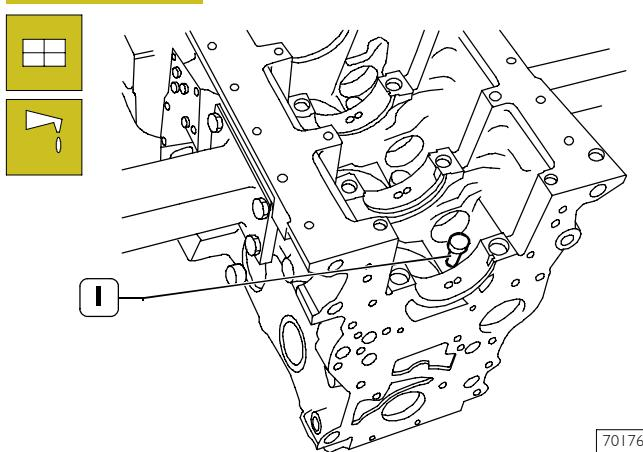
Lubricate the tappets (1) and fit them into the relevant housings on the engine block.
