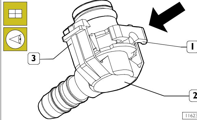
All the low-pressure fuel pipes are fastened with clips shown in the picture.
