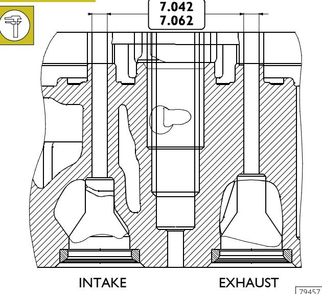
Use a bore dial gauge to measure the inside diameter of the valve guides, the read value shall comply with the value shown in the figure.
