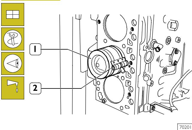
Lubricate accurately the pistons, including the split rings and the cylinder barrel inside.
