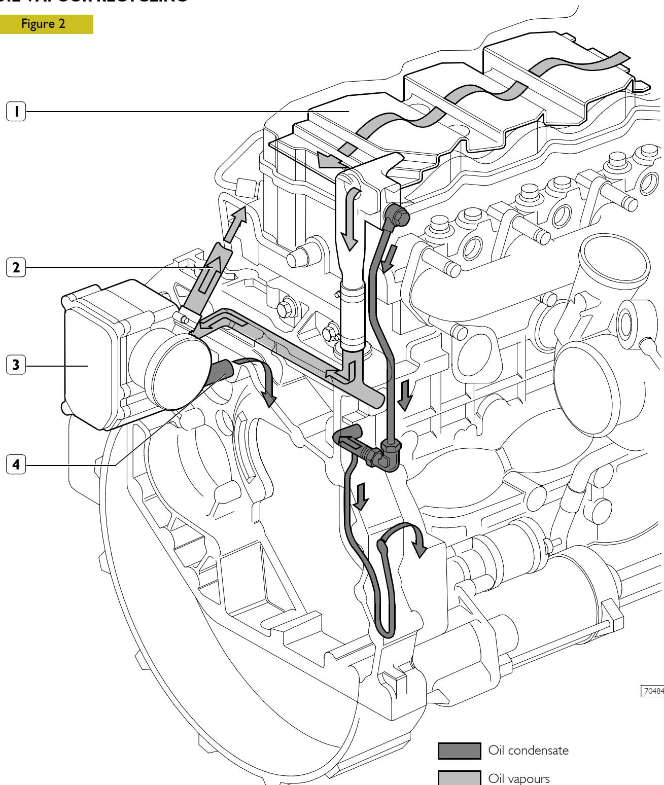
1. Pre-separator - 2. Exhaust to the outside (temporary) - 3. Filter - 4. Return to engine
