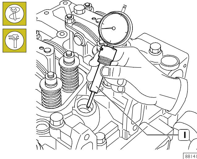
Remove the rocker covers of the 1<sup>st</sup> cylinder; remove the 1<sup>st</sup> injector and place the tool (1) to set the 1<sup>st</sup> cylinder top dead centre position (end-of-compression phase). Pre-load the gauge.
