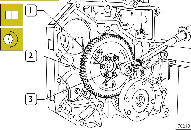
Tighten the screws (1) fastening gear (2) to camshaft (3) to the specified torque.
