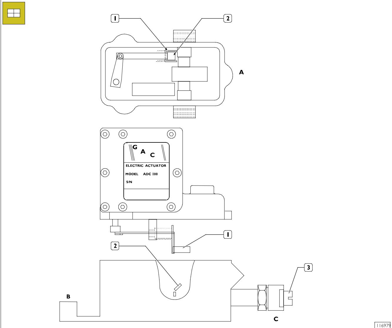
A. The injection pump open seen from above - B. Front (carter side) - C Rear (injector side)
