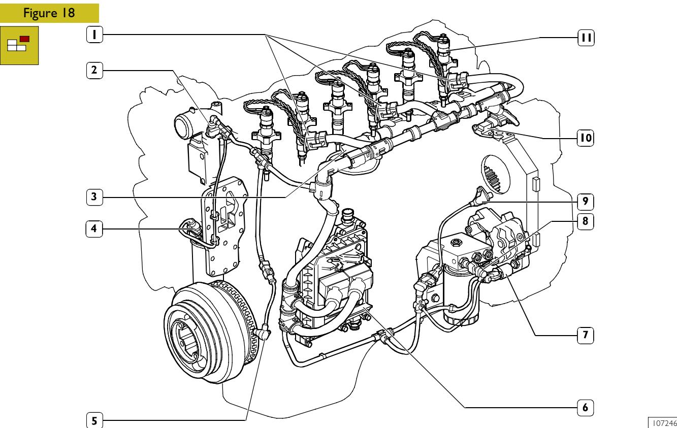
1. Connections for Electro-injectors - 2. Engine cooling liquid temperature's sensor - 3. Cable of the fuel pressure sensor -
