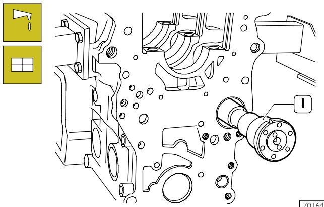
Lubricate the camshaft support bearing and install the camshaft (1) being careful to ensure that the bearing or the shaft support seats are not damaged during the operation.
