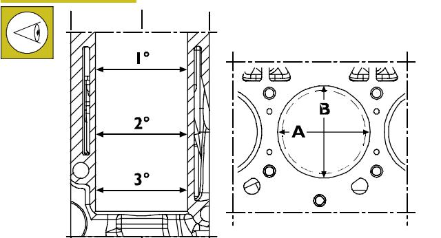
Measurements shall be performed on each cylinder, at three different heights in the barrel and on two planes perpendicular with each other: one parallel to the longitudinal axis of the engine (A), and the other perpendicular (B). Maximum wear is usually found on plane (B) in correspondence with the first measurement.
