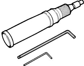
Torque screwdriver for injector solenoid valve connector stop nut setting                 |
