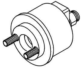
Tool for fitting output shaft front gasket                                 |
