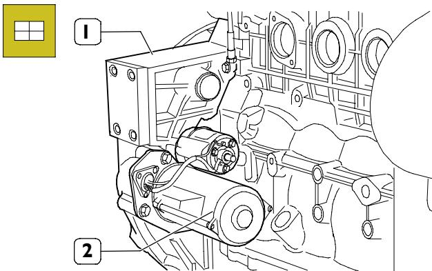
Assemble the starter (2) to the internal part of the flywheel cover.
