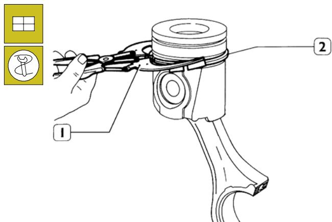
Use pliers 99360183 (1) to fit the split rings (2) on the piston. Split rings shall be fitted with the marking "TOP" facing upwards and their openings shall be displaced with each other by 120°.
