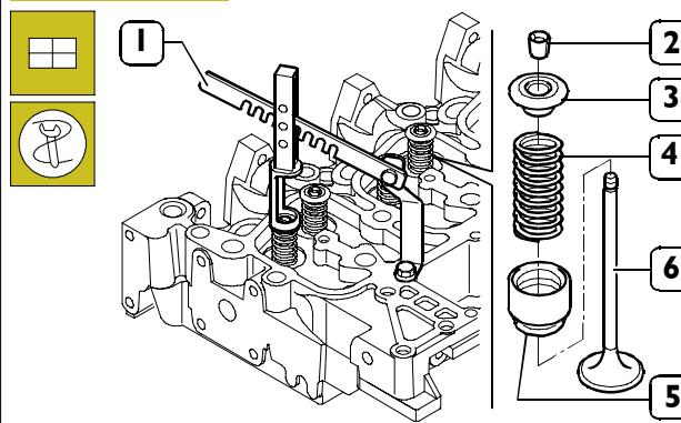
Position on the cylinder head: the spring (4), the upper cap (3); use tool 99360268 (1) to compress the spring (4) and lock the parts to the valve (5) by the cotters (2).
