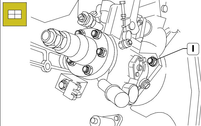
When installing suppli pump on engine, cylinder no.1 must be at TDC, end of compression phase.
