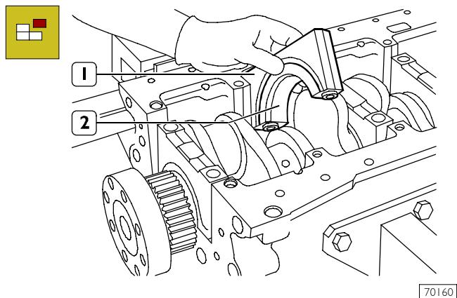
The second last main bearing cap (1) and the relevant support are fitted with shoulder half-bearing (2).
