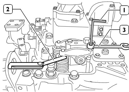
Adjust the play between the rocker arms and valves using a hex key (1), polygonal key (3) and feeler gauge (2).
