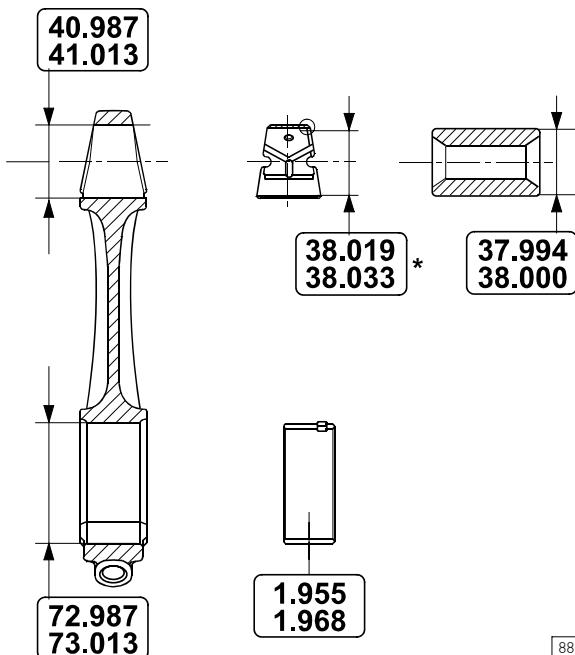
**MAIN DATA FOR CONNECTING ROD, BUSH, PISTON PIN AND HALF BEARINGS**
