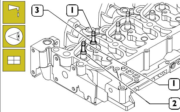
Lubricate the valve stems (1) and fit them into the relevant valve guides according to the position marked at removal.
