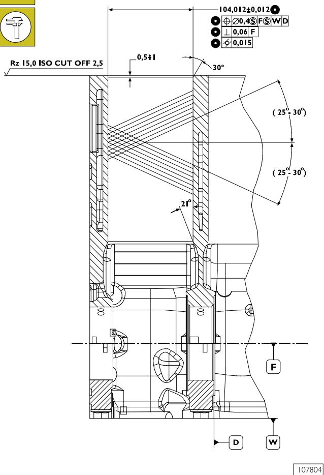
**NOTE** In case of regrinding, all barrels shall have the same oversize (0.4 mm).
