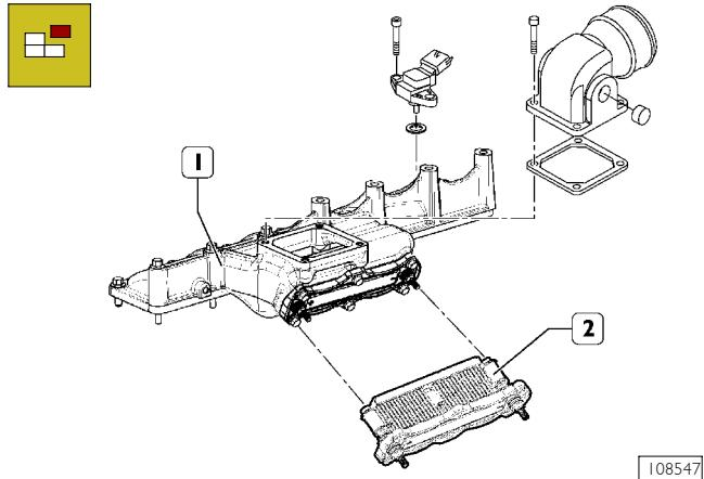
On the opposite side, loosen the fixing screws of the inlet manifold (1) and disassemble the joint to the air heater (2) for the cold start.
