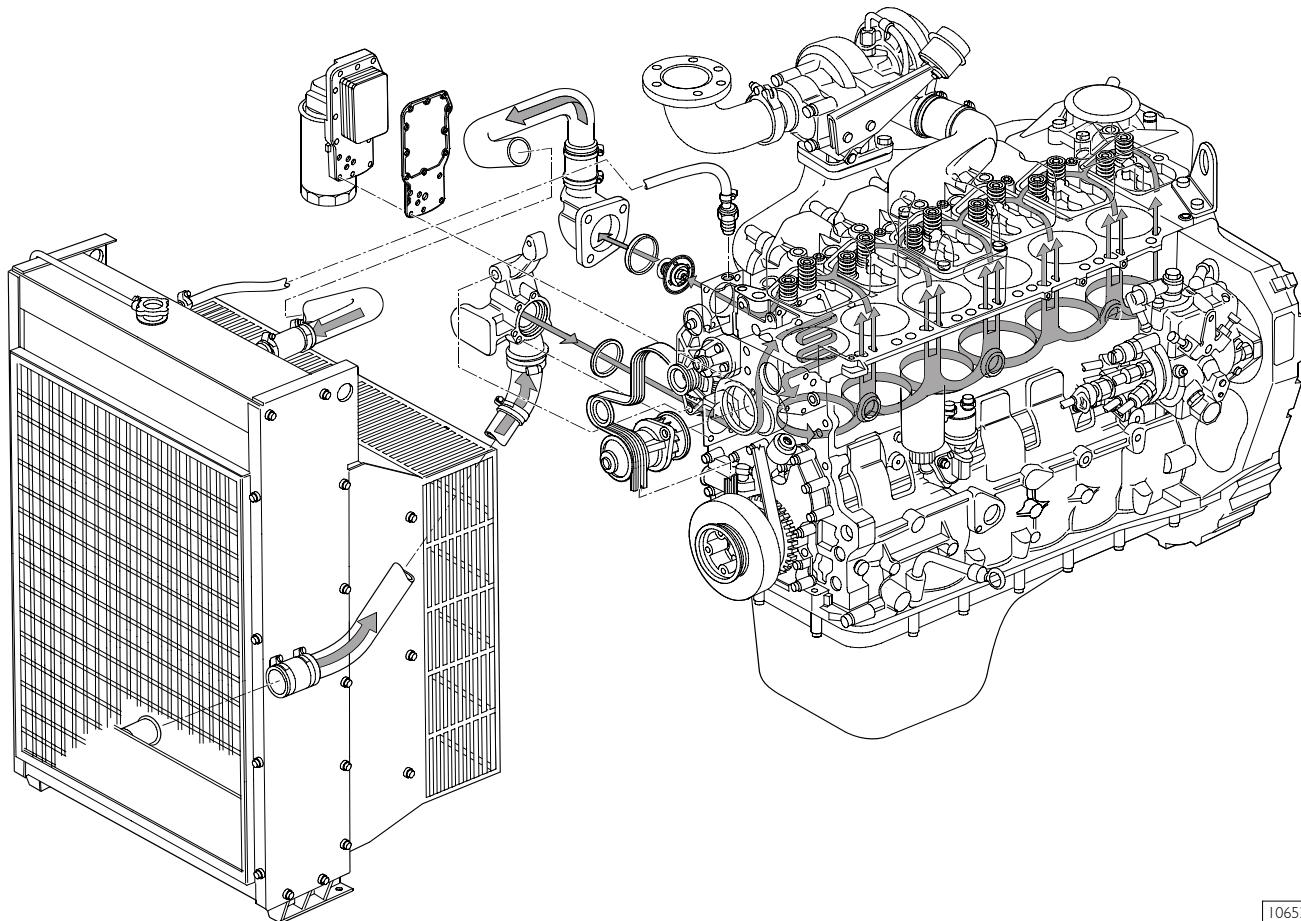
COOLING SYSTEM LAYOUT (6 cyl. engines)
