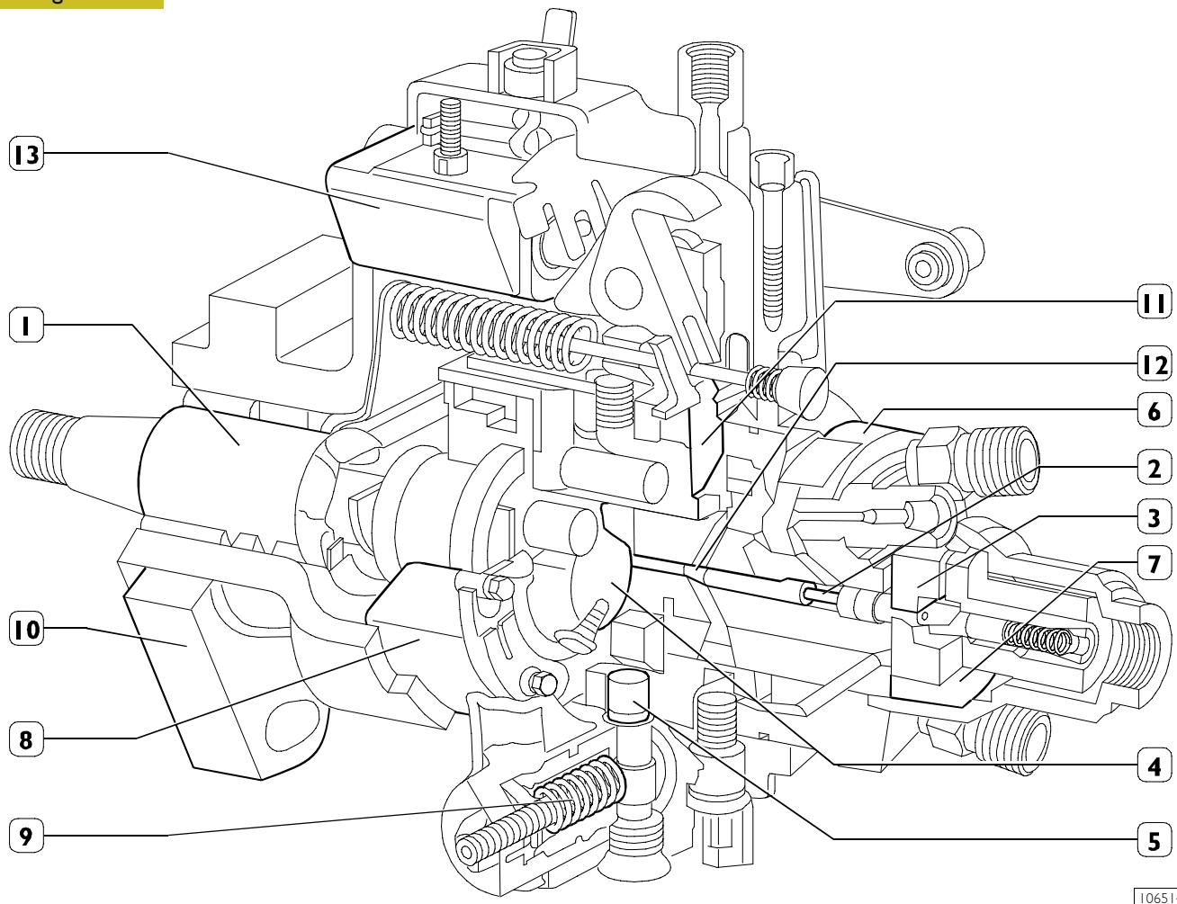
1. Propeller shaft - 2. Timing gear rotor - 3. Transfer pump vanes - 4. Pumping pistons (4) - 5. Cam inner ring - 6. Hydraulic head - 7. Pressure regulator assembly - 8. Regulator - 9. Automatic advance - 10. Seat - 11. Metering valve - 12. Delivery valve - 13. Electric power supply cut-off solenoid.
