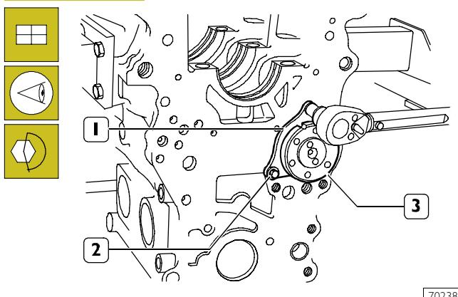
Set camshaft (3) retaining plate (1) with the slot facing the top of the engine block and the marking facing the operator, then tighten the screws (2) to the specified torque.
