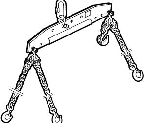
Lifting rig for engine removal/refitting                                 |
