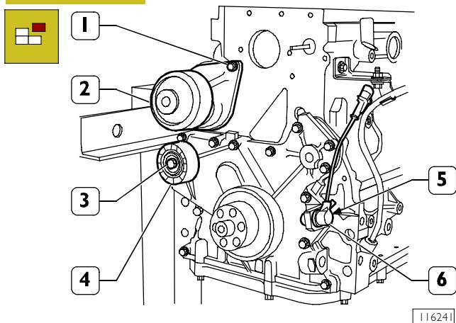
Remove the screws (1) and disconnect the water pump (2). Remove the screw (3) and the roller (4).
