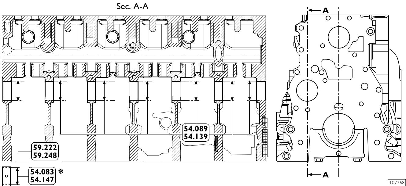
MAIN SPECIFICATIONS OF THE CAMSHAFT BEARING BUSH AND ITS SEAT (6-cylinder engines)
