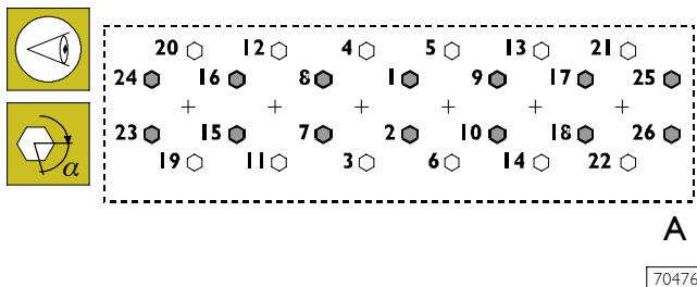
Tightening order layout for cylinder head fastening screws:
