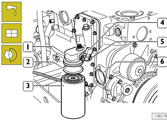
Lubricate the sealing ring (2) with engine oil and set it on the oil filter (3).
