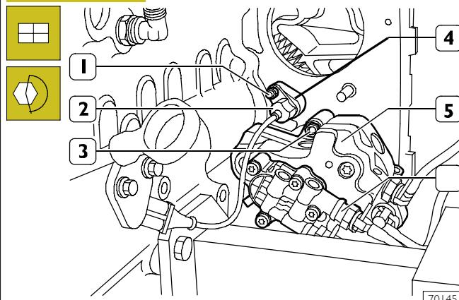
Refit the high pressure pump (6) including the feed pump (5) and tighten the nuts (3) to the specified torque. Fit the support (4) with a new sealing ring, the timing sensor (2) with a new sealing ring and tighten the relevant fastening nut (1) to the specified torque.
