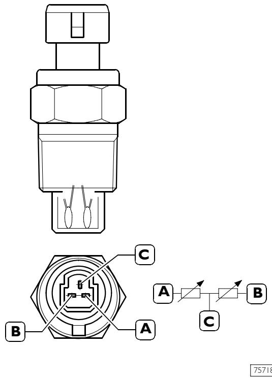
It is a component integrating a temperature sensor. It is assembled to the engine head close to the thermostat unit and its duty is to detect engine cooling liquid temperature.
