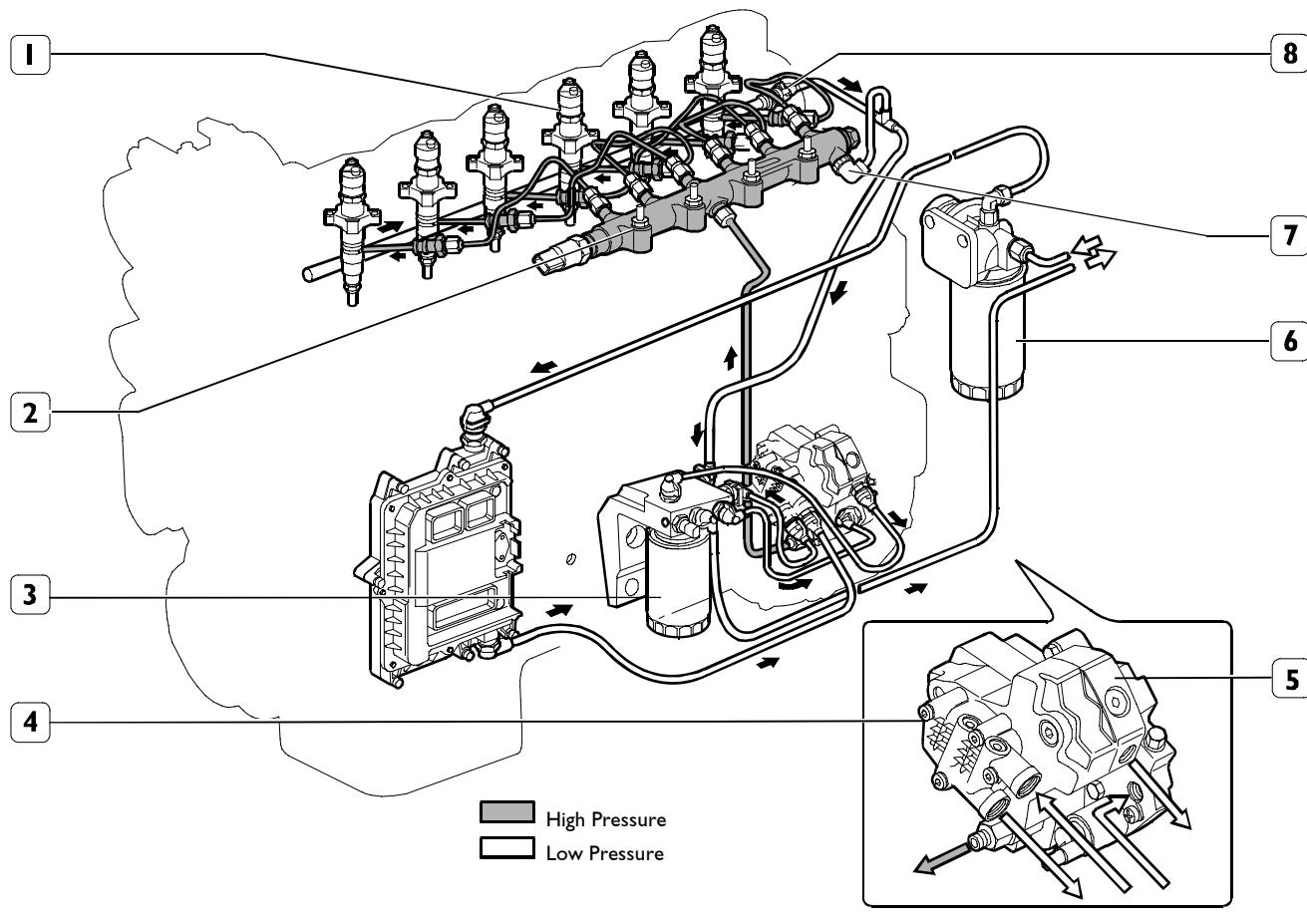
1. Injector - 2. Common Rail - 3. Fuel filter - 4. Mechanical rotor pump - 5. High-pressure pump - 6. Prefilter assembled on chassis - 7. Rail overpressure valve - 8. Pressure limiter for fuel return
