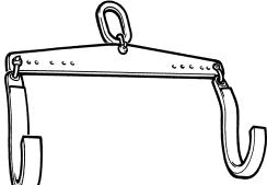
Tool for lifting the output shaft                                         |
