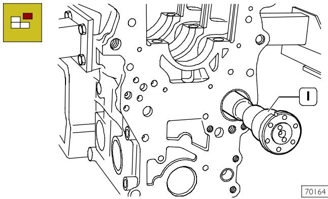
Withdraw carefully the camshaft (1) from the engine block.
