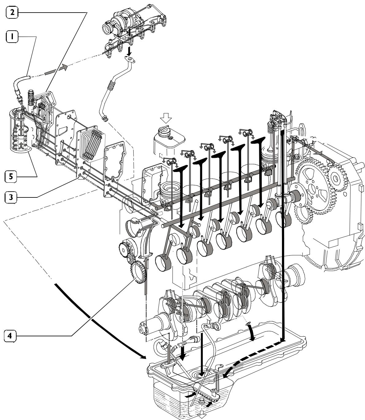
**LUBRICATION SYSTEM LAYOUT (6 cylinder engines)**
