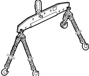
Lifting rig for engine removal/refitting                                |
