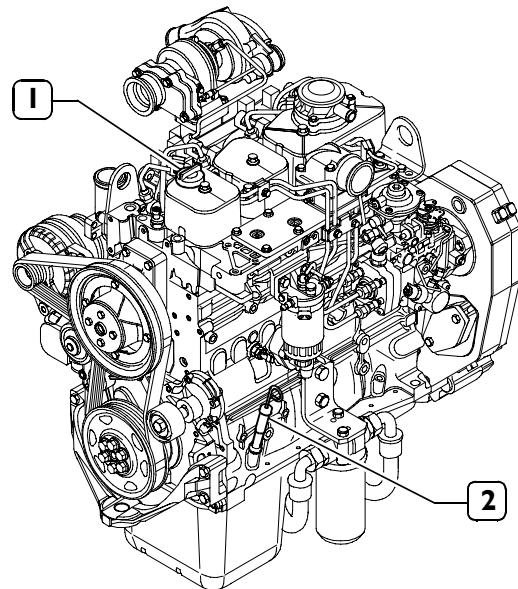
To provide filling, operate through the upper top (1) or through the lateral top (2). During filling operation, the tops must be removed as well as the rod in order to make the oil flow easier".
