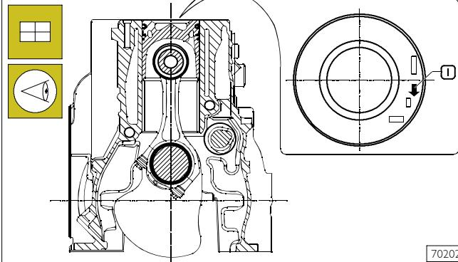
DIAGRAM FOR CONNECTING ROD-PISTON ASSEMBLY FITTING INTO BARREL
