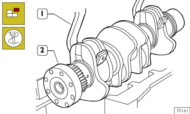
Use tool 99360500 (1) and hoist to remove the output shaft (2) from the block.
