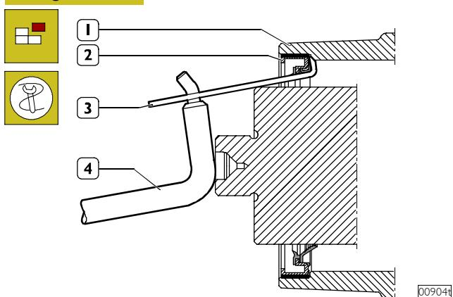
Using the specific tie rod (3) of the tool 99363204 and the ancillary lever (4), remove the external holding ring (2) from the front cover (1).
