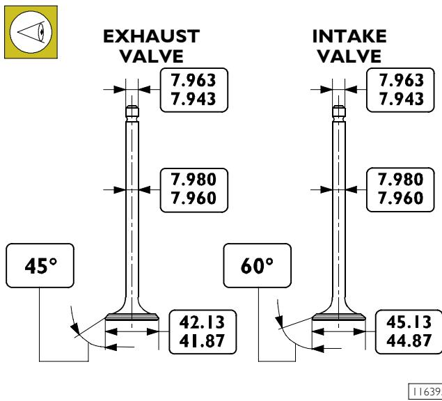
INTAKE AND EXHAUST VALVE MAIN DATA
