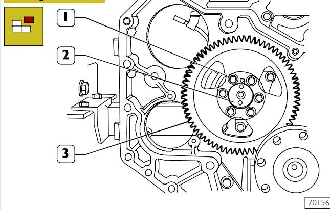
Remove the screws (1) and remove the gear (3) from the camshaft (2).
