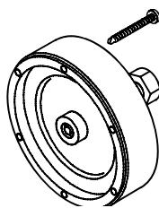
Tool to remove output shaft rear gasket
