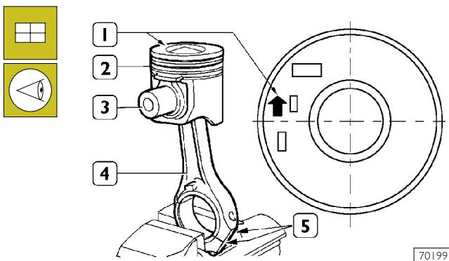
Connect piston (2) to connecting rod (4) with pin (3) so that the reference arrow (1) for fitting the piston (2) into the cylinder barrel and the numbers (5) marked on the connecting rod (5) are read as shown in the figure.
