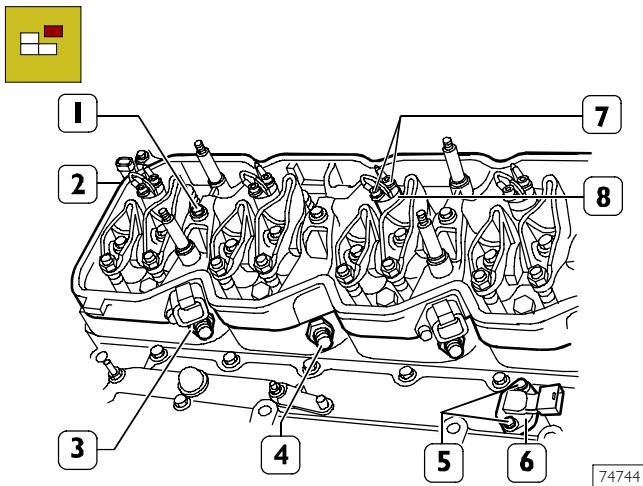
Remove nuts (7) and disconnect the electrical cables from injectors (8).
