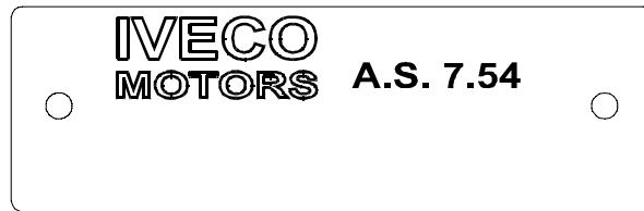
In case the FPT tag is not present because it is a motor with an injection pump that has a setting of 50 Hz, it is necessary to proceed in the application of a tag in the illustrated area as in Figure 4 stamping it as the figure example.
