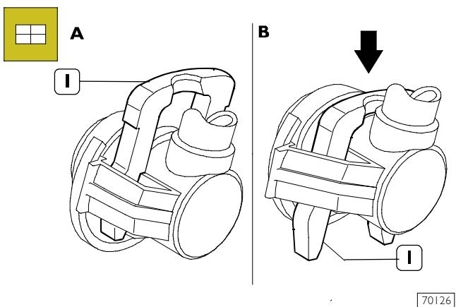
**NOTE** To connect fuel pipelines (3 and 4, Figure 116) in low pressure from the relating connection unions it is necessary to press the locking fastener (1) as shown in picture B.
