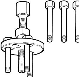
Injection pump gear extractor.                                               |
