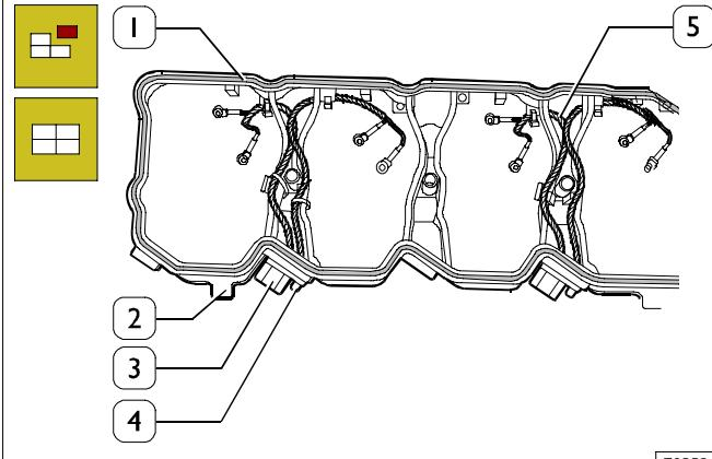
Check electrical cable (5) conditions, replace if damaged by cutting the support (2) clamps and removing the screws (4) that secure it to connections (3).
