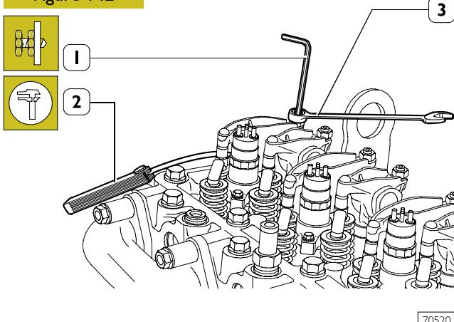
Adjust clearance between rockers and valves using setscrew wrench (1), box wrench (3) and feeler gauge (2).
