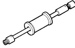
Tool to remove injectors                                                   |
