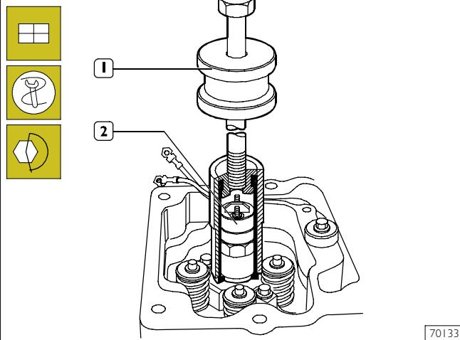
Use tool 99342101 (1) to fit the injector (2) into its seat.
