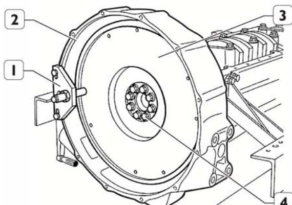
Remove two opposite screws (1) from the area where the withdrawal pins will be introduced (2, Figure 41).
