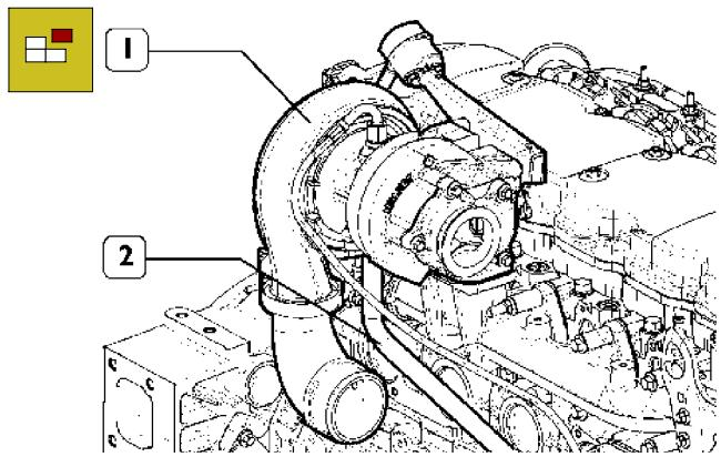
Remove the screws and remove the oil pipe (1) from the turbocharger pipe (2) and from the engine block.
