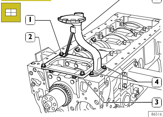
Fit the plate (3), the oil pick up tube (5) and tighten the fastening screws (1, 2, 4) to the specified torque.
