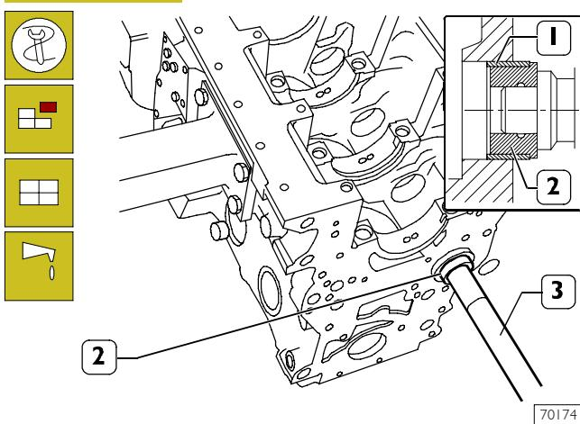
To replace the bearing (1) use tool 99360362 (2) and handle 99370006 (3) to remove and install it.
