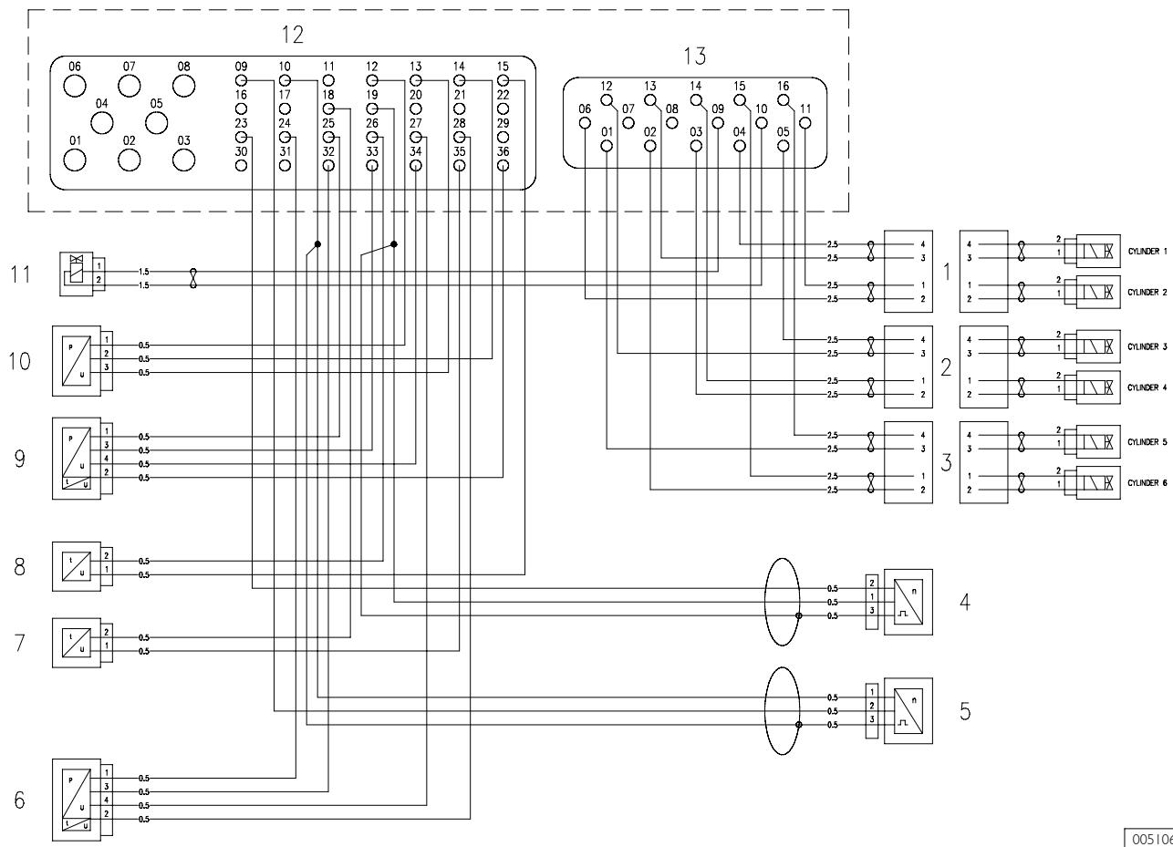
1. Injectors for cylinders 1-2 - 2 Injectors for cylinders 3-4 - 3. Injectors for cylinders 5-6 - 4. Engine rpm sensor -
