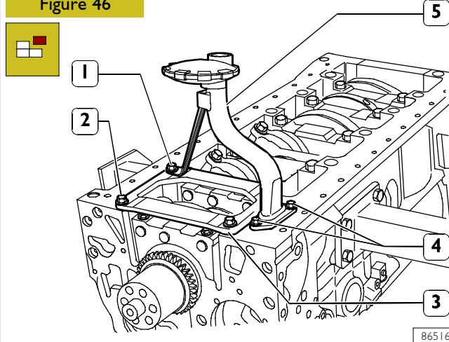
Remove the screws (1 and 4) and disassemble the oil suction tube (5). Remove the screws (2) and disassemble the stiffening plate (3).
