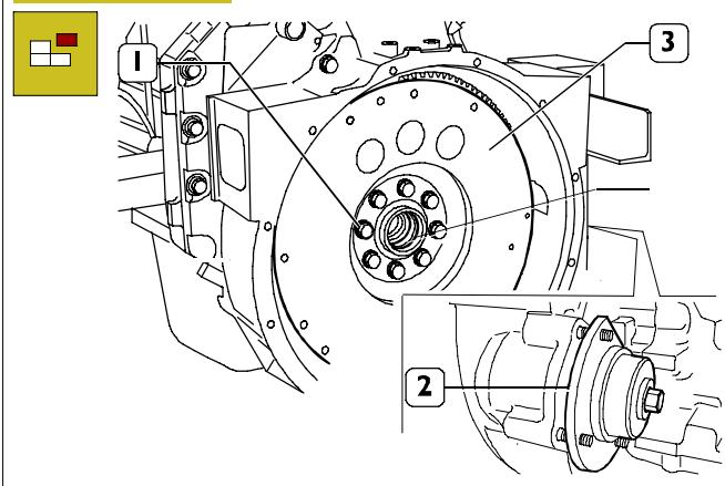
Remove two opposite screws (1) from the area where the withdrawal pins will be introduced (2, Figure 41).
