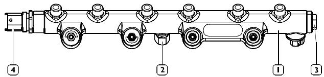
1. Rail – 2. Fuel inlet from high-pressure pump –
