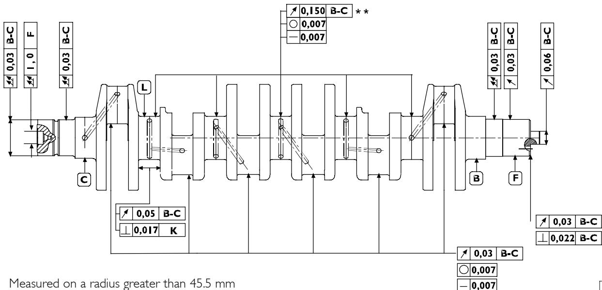
MAIN OUTPUT SHAFT TOLERANCES
