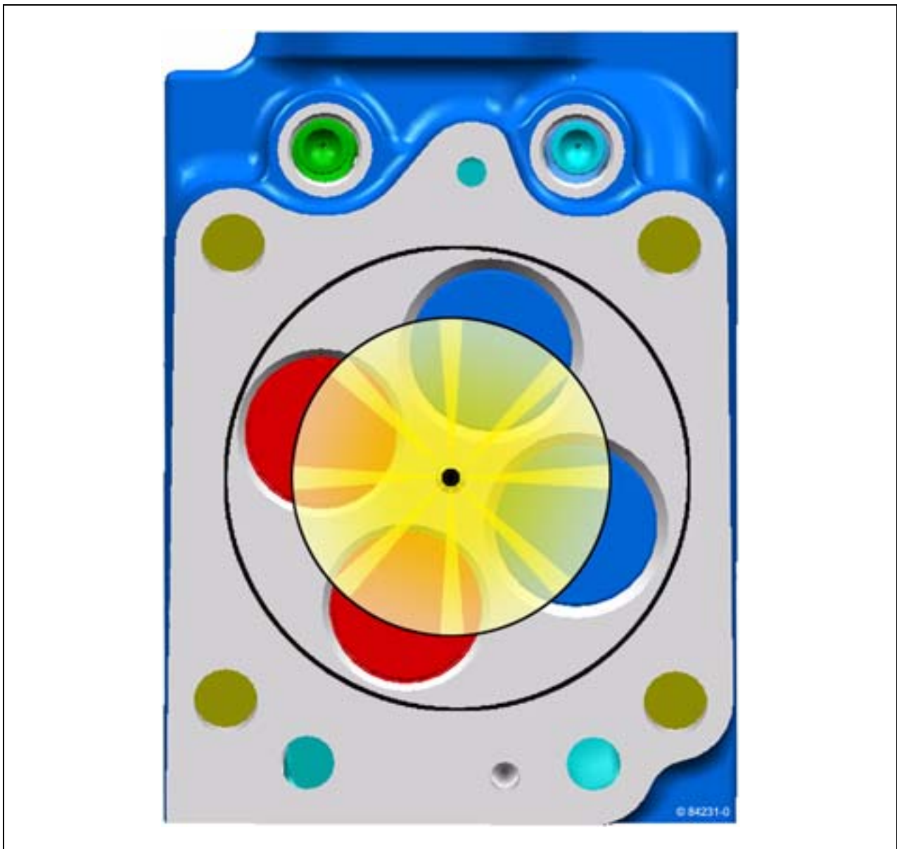
Figure 2-21 Spray behavior of the multi-hole nozzle
