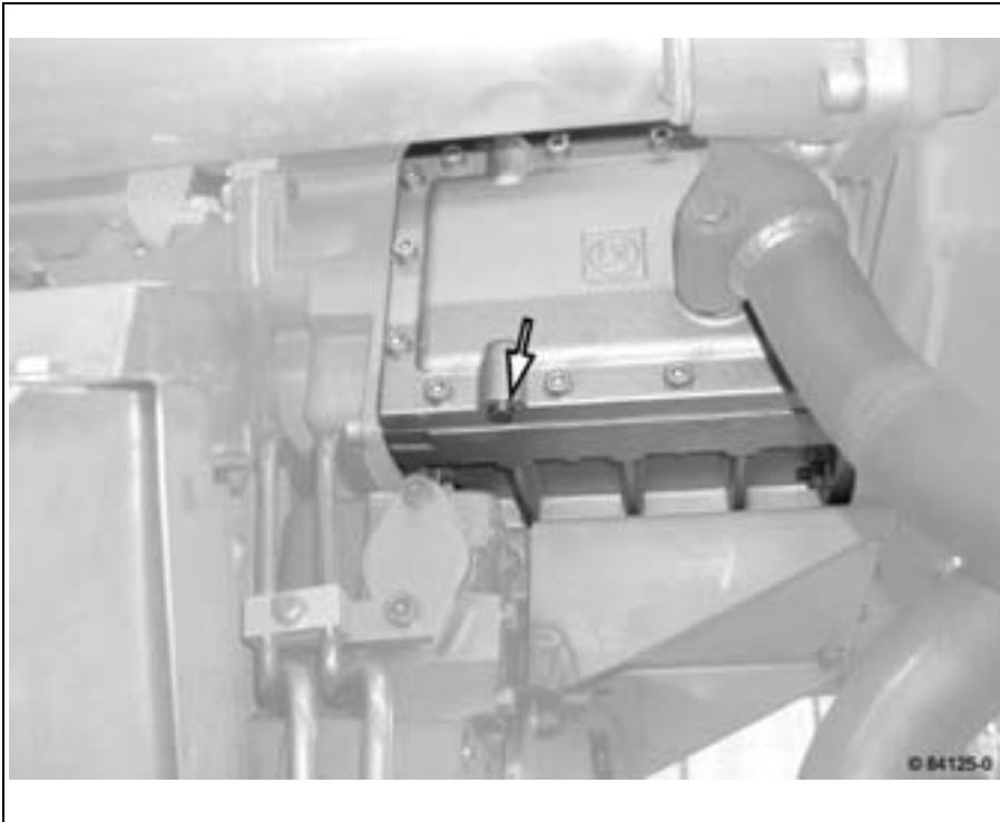
Figure 7 Charge air cooler on the damper side (free side)
