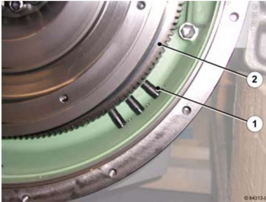
Figure 2-27 Frequency pick-up (installation example for EMR2)
