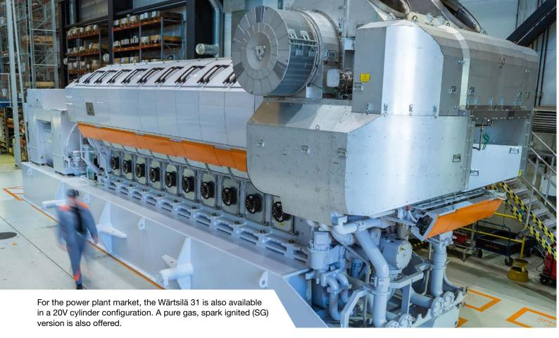
In the cruise and ferry sector, the Wärtsilä 31 represents a particularly good investment for ferry and Ro-Pax fleet operators focusing on trimming their fuel expenses while maintaining high standards in environmental performance. Within the merchant fleet, the Wärtsilä 31 is designed for application as a main engine for small to medium sized tankers, bulk carriers, and container vessels.
