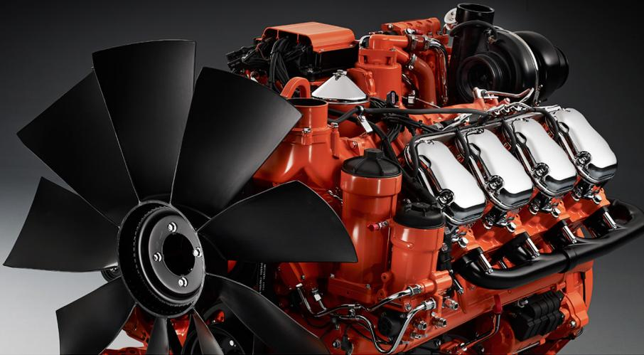
The engines for power generation from Scania are based on a robust design with a strength optimised cylinder block containing wet cylinder liners that can easily be exchanged. Individual cylinder heads with 4 valves per cylinder promotes reparability and fuel economy.
